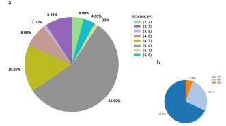
Fig. 10 (a) Percentage of unique Li $^+$  solvation structures in mixed carbonate 1:1 EC/DEC + 1 M LiPF $_6$  electrolyte. The Li $^+$  is surrounded by EC, DEC, PF $_6$  $^-$ . A value of PF $_6$  = 0 indicates that the PF $_6$  $^-$  anion is located outside the primary solvation shell (SSIPs). Inside the primary solvation shell, PF $_6$  = 1 refers to CIPs, and PF $_6$  > 1 refers to AGGs. (b) Percentage of SSIPs, CIPs, and AGGs.
