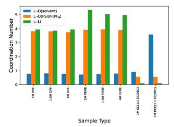
**Fig. 8** Atomic coordination numbers of the electrolytes. The CN of Li<sup>+</sup> – Li<sup>+</sup> and Li<sup>+</sup>–F(PF<sub>6</sub><sup>-</sup>) in mixed EC/DEC carbonate electrolyte is assumed to be the same for both EC and DEC solvents.
