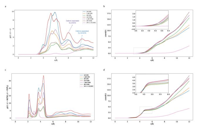
Fig. 7 (a) RDFs of  $Li^+-Li^+$  and corresponding (b) coordination numbers as a function of distance. (c) RDFs of  $Li^+-N(FSI^-)$ ,  $Li^+-P(PF_6^-)$ , and corresponding (d) coordination numbers as a function of distance.
