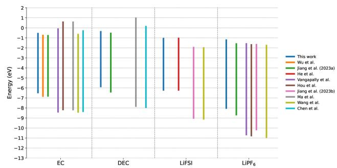
Fig. 3 DFT validation of HOMO/LUMO energy levels of the studied salts and solvents. This work, Wu *et al.*, <sup>57</sup> Jiang *et al.* (2023a), <sup>58</sup> and He *et al.* <sup>59</sup> used the PBE functional in VASP, while Vangapally *et al.*, <sup>60</sup> Hou *et al.*, <sup>61</sup> Jiang *et al.* (2023b), <sup>62</sup> Ma *et al.*, <sup>63</sup> Wang *et al.*, <sup>64</sup> and Chen *et al.* <sup>65</sup> used the B3LYP functional in Gaussian software.
