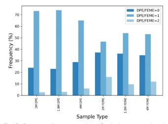
Fig. 12 Frequency of occurrence of the Li<sup>+</sup> solvation structures in each fluorinated electrolyte based on the presence of zero, one, and two solvent molecules
