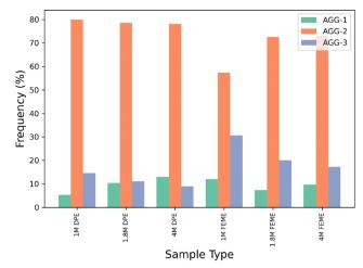
Fig. 11 Detailed speciation of AGG in each fluorinated electrolyte with the frequency of occurrence. AGG-1 (one and two FSI- anions), AGG-2 (three and four FSI<sup>-</sup> anions), and AGG-3 (five and six FSI<sup>-</sup> anions)
