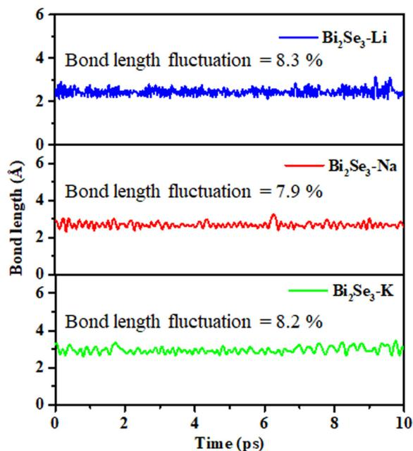
Fig. 8 Fluctuation in the bond length of Li/Na/K atoms in Li/Na/K–Bi<sub>2</sub>Se<sub>3</sub> at 400 K.
