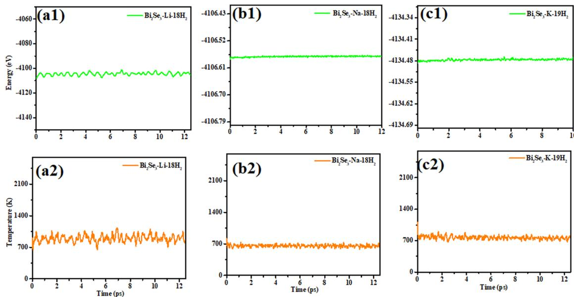
Fig. 7 MD simulation visualizations for the  $18\text{H}_2$ ,  $18\text{H}_2$ , and  $19\text{H}_2 + \text{Li/Na/K-Bi}_2\text{Se}_3$  systems at 906 K, 821 K, and 1112 K. The outcomes demonstrate the changes in total energy (a1)–(c1) and temperature (a2)–(c2) over time (ps).
