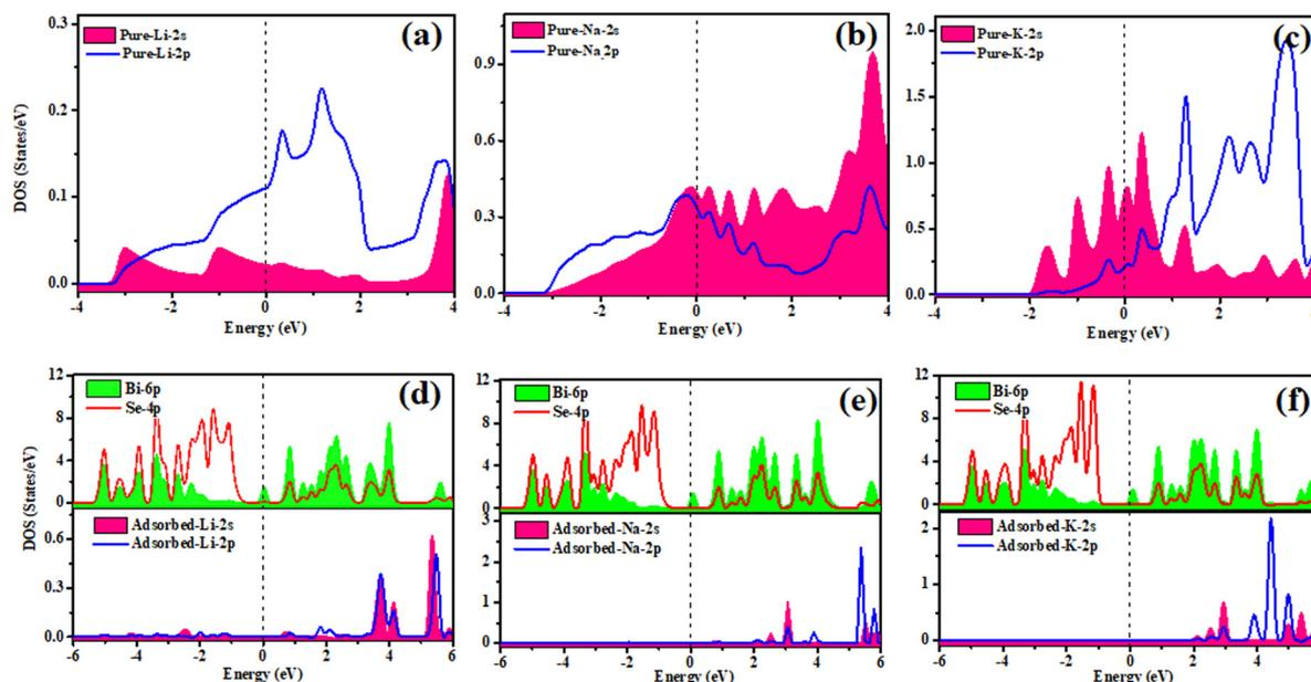
Fig. 3 Projected density of states (PDOS) for unbound (a) pure Li, (b) Na, and (c) K and adsorbed (d)  $\text{Bi}_2\text{Se}_3$ -Li, (e)  $\text{Bi}_2\text{Se}_3$ -Na, and (f)  $\text{Bi}_2\text{Se}_3$ -K.
