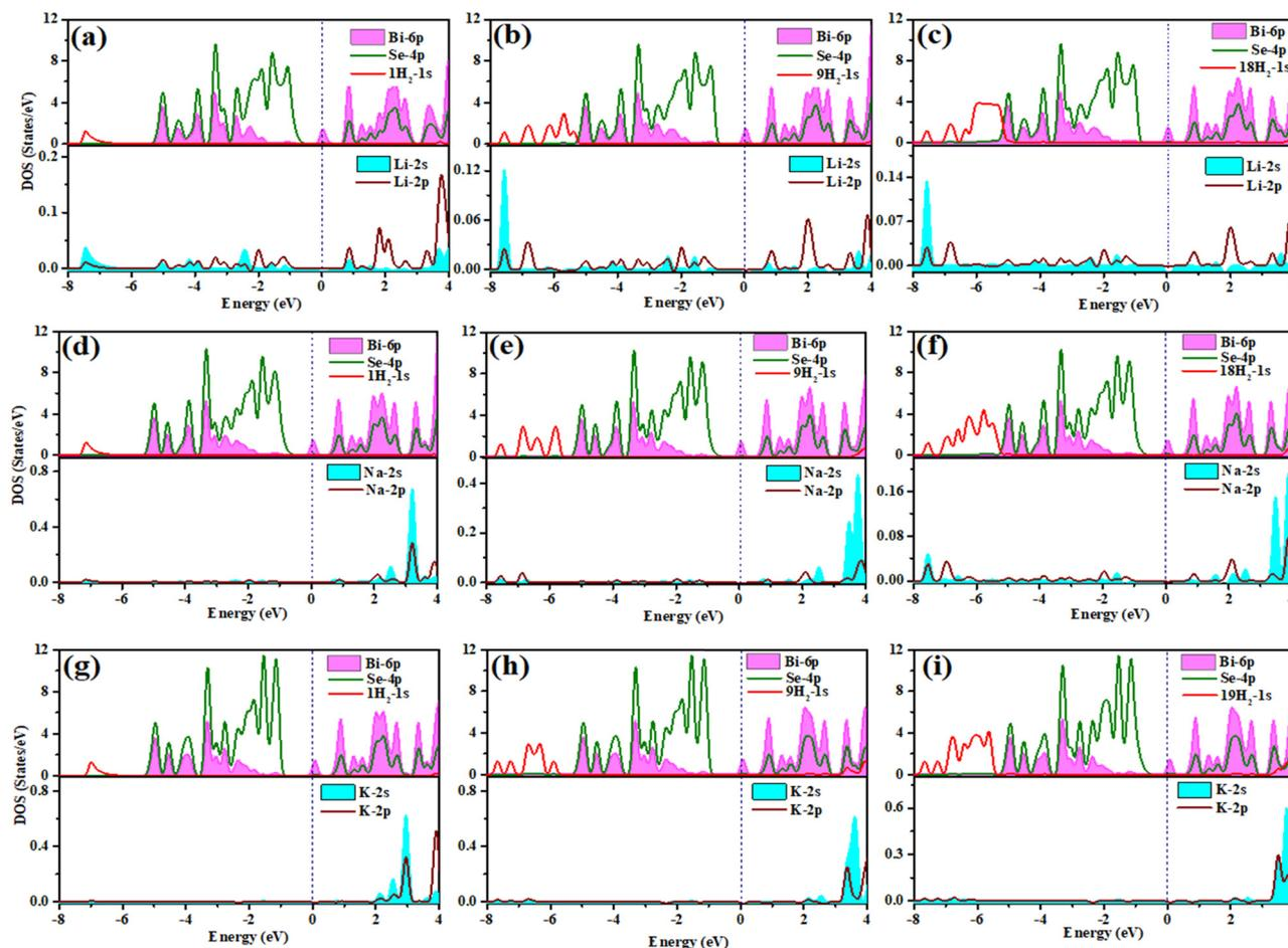
Fig. 5 Projected density of states (PDOS) for (a)  $\text{Bi}_2\text{Se}_3\text{-Li-1H}_2$ , (b)  $\text{Bi}_2\text{Se}_3\text{-Li-9H}_2$ , (c)  $\text{Bi}_2\text{Se}_3\text{-Li-18H}_2$ , (d)  $\text{Bi}_2\text{Se}_3\text{-Na-1H}_2$ , (e)  $\text{Bi}_2\text{Se}_3\text{-Na-9H}_2$ , (f)  $\text{Bi}_2\text{Se}_3\text{-Na-18H}_2$ , (g)  $\text{Bi}_2\text{Se}_3\text{-K-1H}_2$ , (h)  $\text{Bi}_2\text{Se}_3\text{-K-9H}_2$ , and (i)  $\text{Bi}_2\text{Se}_3\text{-K-19H}_2$ .
