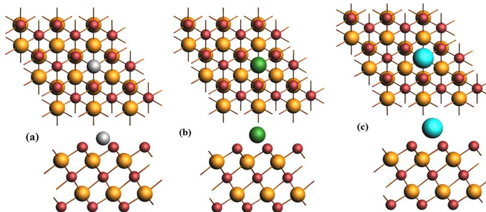
Fig. 2 Views of optimized configurations of (a) Li-, (b) Na- and (c) K-modified  $\text{Bi}_2\text{Se}_3$ .
