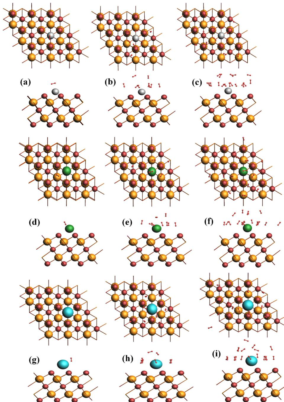
Fig. 4 Optimized geometry of Li-Bi<sub>2</sub>Se<sub>3</sub>: (a) 1H<sub>2</sub>, (b) 9H<sub>2</sub>, (c) 18H<sub>2</sub>, Na-Bi<sub>2</sub>Se<sub>3</sub>, (d) 1H<sub>2</sub>, (e) 9H<sub>2</sub>, (f) 18H<sub>2</sub>, K-Bi<sub>2</sub>Se<sub>3</sub>, (g) 1H<sub>2</sub>, (h) 9H<sub>2</sub> and (i) 19H<sub>2</sub>.
