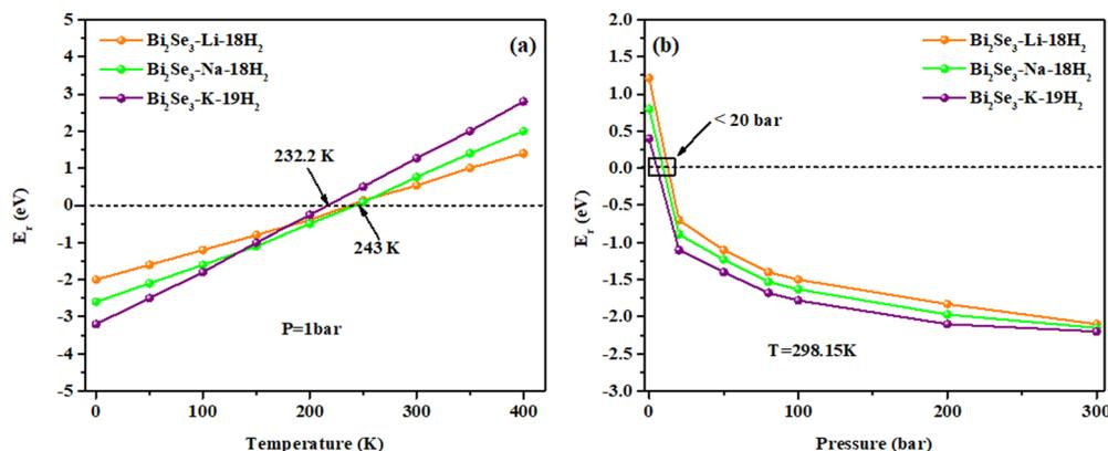
Fig. 9 (a) Temperature-dependent behavior of  $E_r$  for the adsorption of  $n\text{H}_2$  molecules on Li/Na/K–Bi<sub>2</sub>Se<sub>3</sub>-decorated surfaces under standard atmospheric pressure (1 bar). (b) Pressure-dependent variation in  $E_r$  for  $\text{H}_2$  adsorption on Li/Na/K–Bi<sub>2</sub>Se<sub>3</sub>-decorated surfaces at a fixed temperature of 298 K.
