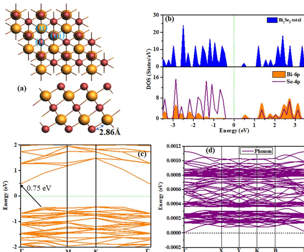
Fig. 1 (a) Z and X-views of the optimized structure of pure Bi<sub>2</sub>Se<sub>3</sub>. (b) Partial density of states (PDOS), (c) band structure, and (d) phonon dispersion curves.
