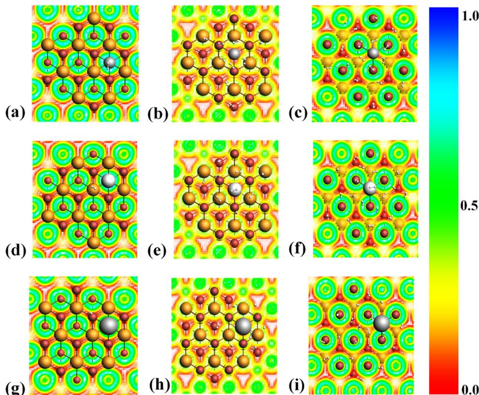
Fig. 6 ELF (a) 1H<sub>2</sub>, (b) 9H<sub>2</sub>, and (c) 18H<sub>2</sub> represent Li-decorated Bi<sub>2</sub>Se<sub>3</sub>; (d) 1H<sub>2</sub>, (e) 9H<sub>2</sub>, and (f) 18H<sub>2</sub> correspond to Na-decorated Bi<sub>2</sub>Se<sub>3</sub>; and (g) 1H<sub>2</sub>, (h) 9H<sub>2</sub>, and (i) 19H<sub>2</sub> represent K-decorated Bi<sub>2</sub>Se<sub>3</sub>.
