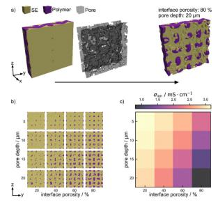
Fig. 3 (a) Introduction of interfacial porosity into the virtual microstructure. (b) Top-view images of the virtual microstructures with varying pore depths and interface porosity. (c) Ionic conductivity as a function of pore depth and interface porosity for the infiltrated mesh structure.
