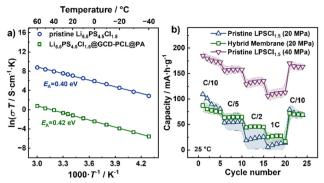
Fig. 4 (a) Arrhenius plot of the infiltrated membrane LPSCl<sub>1.5</sub>@GCD–PCL@PA with activation energy  $E_{\rm A}=0.42$  eV and pristine LPSCl<sub>1.5</sub> with activation energy  $E_{\rm A}=0.40$  eV. (b) Discharge capacities of the rate-performance test in a Li/In half-cell setup at 20 MPa and 40 MPa, where 1C = 180 mAh g<sup>-1</sup>.
