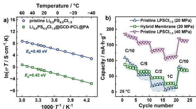
Fig. 4 (a) Arrhenius plot of the infiltrated membrane  $\text{LPSCl}_{1.5}@\text{GCD-PCL}@\text{PA}$  with activation energy  $E_A = 0.42$  eV and pristine  $\text{LPSCl}_{1.5}$  with activation energy  $E_A = 0.40$  eV. (b) Discharge capacities of the rate-performance test in a Li/In half-cell setup at 20 MPa and 40 MPa, where  $1\text{C} = 180$   $\text{mAh g}^{-1}$ .
