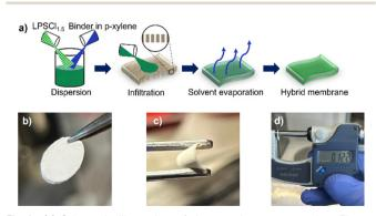
Fig. 1 (a) Schematic illustration of the membrane preparation. Photographs showing (b) an infiltrated membrane, (c) a bent, infiltrated membrane, and (d) thickness measurement, showing the membrane thickness in mm.
