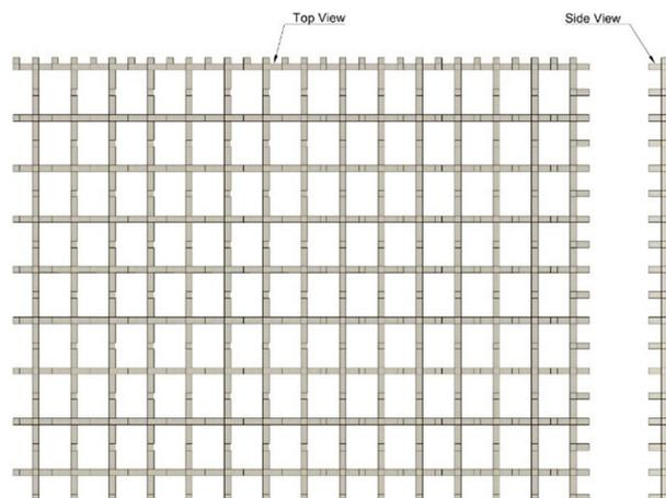
**Fig. 2** Top and side view schematic of the 3D-printed spacer inserted in the negative half-cell. The top view illustrates the open-grid design used to form localized cavities for iron deposition. The side view shows the spacer's position relative to the carbon fabric and membrane.
