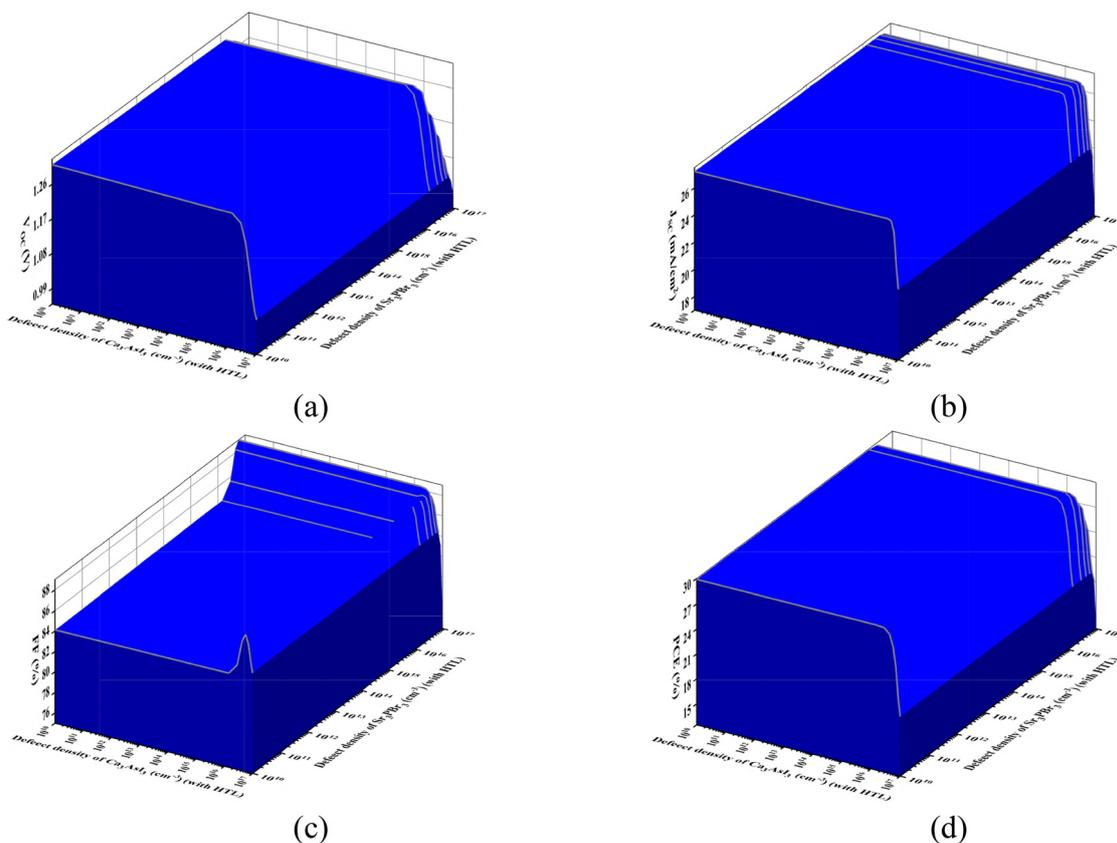
Fig. 7 Impact of defect density variation in  $\text{Sr}_3\text{PbBr}_3$  and  $\text{Ca}_3\text{AsI}_3$  (device-iv) on the photovoltaic parameters, (a)  $V_{\text{OC}}$ , (b)  $J_{\text{SC}}$ , (c) FF, and (d) PCE.
