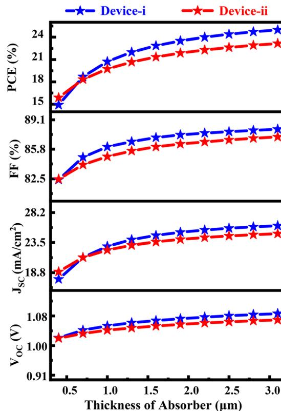
Fig. 2 Impact of the thickness variation of Sr<sub>3</sub>PBr<sub>3</sub> (device-i) and Ca<sub>3</sub>AsI<sub>3</sub> (device-ii) on photovoltaic parameters.
