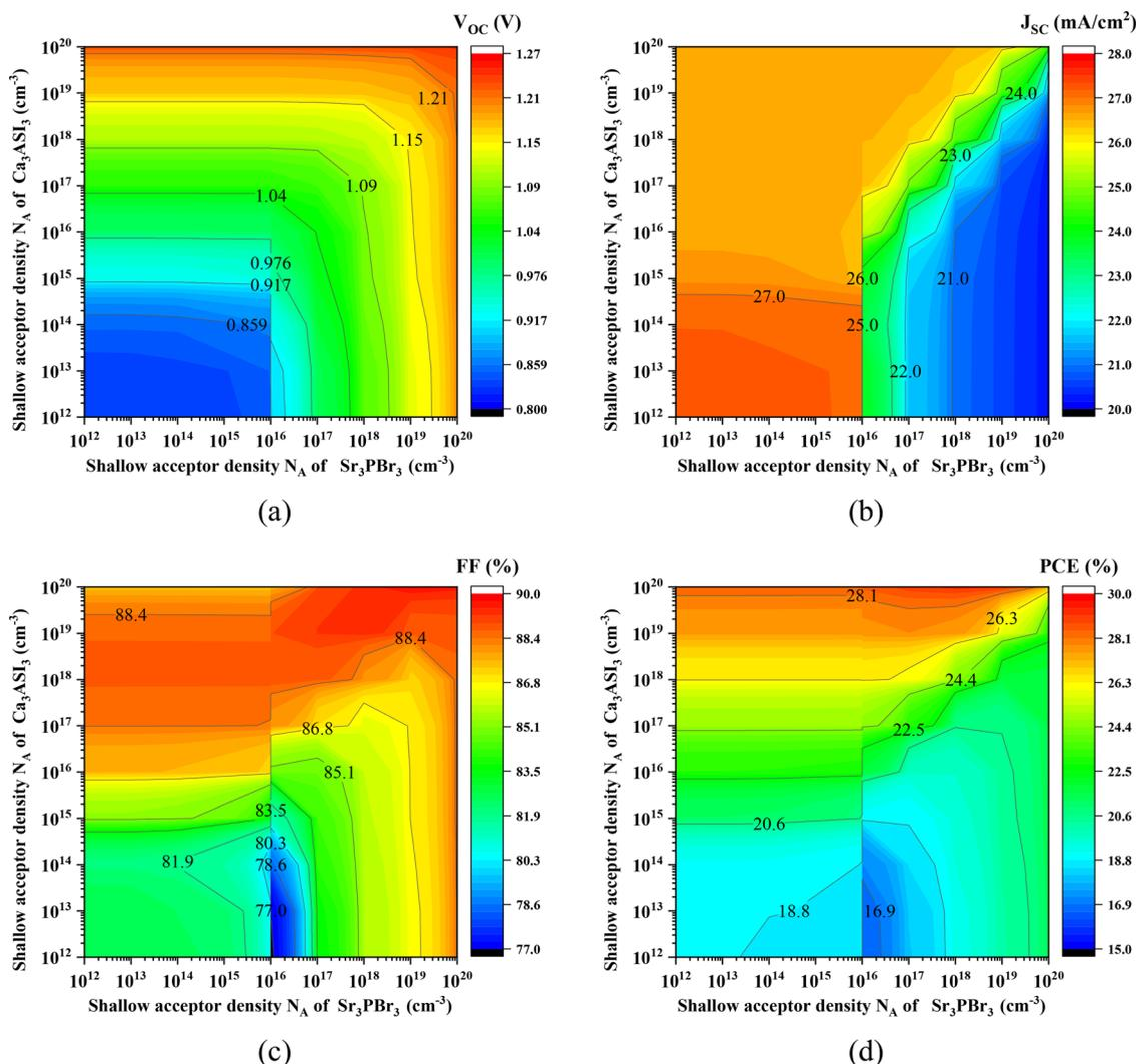
Fig. 9 Role of shallow acceptor density variation in  $\text{Sr}_3\text{PbBr}_3$  and  $\text{Ca}_3\text{AsI}_3$  (device-iii) on the photovoltaic parameters, (a)  $V_{\text{OC}}$ , (b)  $J_{\text{SC}}$ , (c) FF, and (d) PCE.
