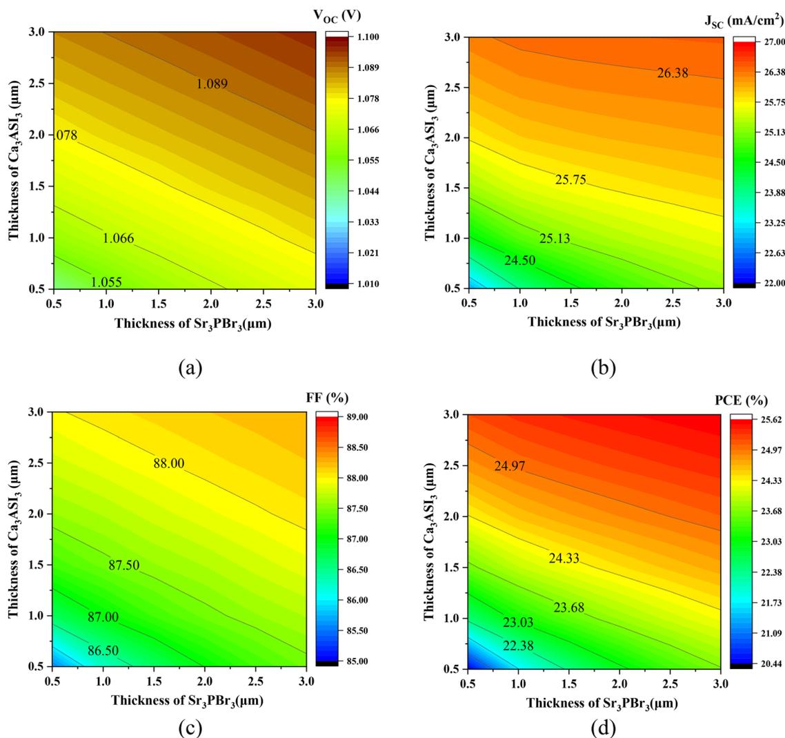
Fig. 3 Role of thickness variation of Sr<sub>3</sub>PbBr<sub>3</sub> and Ca<sub>3</sub>AsI<sub>3</sub> (device-iii) on the photovoltaic parameters, (a)  $V_{OC}$ , (b)  $J_{SC}$ , (c) FF, and (d) PCE.
