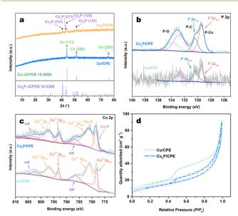
Fig. 2 (a) XRD patterns of Co/CPE and Co<sub>2</sub>P/CPE. (b) P 2p and (c) Co 2p XPS spectra of Co/CPE and Co<sub>2</sub>P/CPE. (d) N<sub>2</sub> adsorption-desorption isotherms of Co/CPE and Co<sub>2</sub>P/CPE
