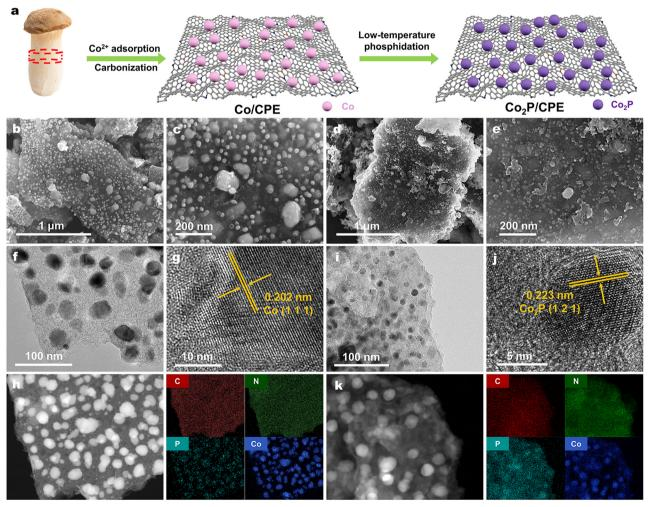
Fig. 1 (a) Schematics of the preparation process of Co<sub>2</sub>P/CPE cocatalysts. Low- and high-magnification SEM images of (b) and (c) Co/CPE and (d) and (e) Co<sub>2</sub>P/CPE. TEM and HRTEM images (f) and (g) Co/CPE and (i) and (j) Co<sub>2</sub>P/CPE. HAADF-STEM images and the corresponding EDX elemental mapping images of (h) Co/CPE and (k) Co<sub>2</sub>P/CPE.
