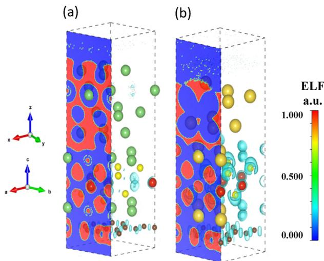
Fig. 7 Electron localization function (ELF) plots at full adsorption capacity for (a) Li- $\text{VS}_2/\text{Gr}$  and (b) Na- $\text{VS}_2/\text{Gr}$  heterostructures. Red regions indicate high electron localization (electron-rich zones), while blue regions correspond to low localization (electron-depleted zones). The left panels display ELF isosurfaces, and the right panels show the corresponding atomic configurations.
