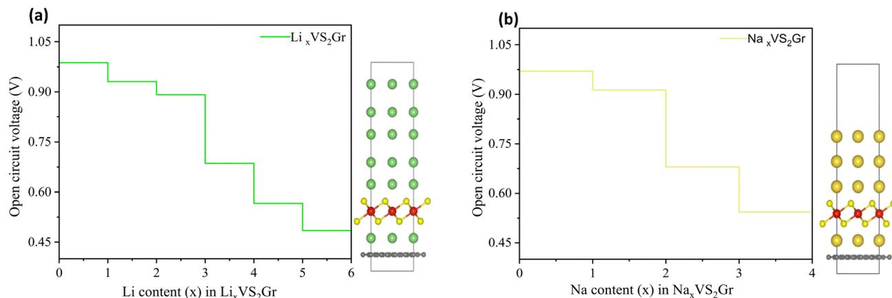
Fig. 10 Computed voltage profile of (a) Li-intercalated VS<sub>2</sub>/Gr relative to Li/Li<sup>+</sup> and (b) Na-intercalated VS<sub>2</sub>/Gr relative to Na/Na<sup>+</sup>.
