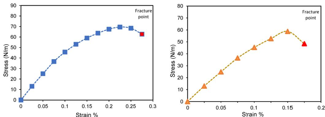
Fig. 5 The uniaxial stress–strain behavior of the VS<sub>2</sub>/Gr composite when subjected to tensile strain along the armchair and zigzag orientations.
