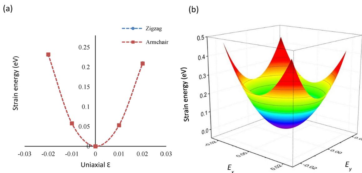
Fig. 4 Structural and mechanical response of the 2D  $\text{VS}_2/\text{Gr}$  composite under uniform expansion: (a) uniaxial strain energy-strain curves along the armchair and zigzag directions and (b) 3D fitted surface plot of total energy as a function of elastic strain.
