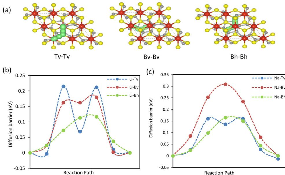
Fig. 9 (a) Diffusion pathways of Li<sup>+</sup>/Na<sup>+</sup> across the outer layer and interlayer regions of VS<sub>2</sub>/graphene. (b) and (c) Energy barrier profiles for Li and Na ion diffusion across the three evaluated pathways.
