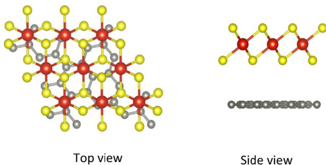
Fig. 2 Diagram of the composite configuration of the VS<sub>2</sub>/Gr composite structure. The gray, blue, red, and yellow spheres correspond to carbon (C), vanadium (V), and sulfur (S) atoms, respectively.
