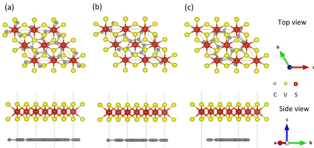
Fig. 1 Top and side views of the three interfacial stacking configurations of the VS<sub>2</sub>/graphene heterobilayer: (a) AA stacking, (b) AB stacking, and (c) BA stacking.
