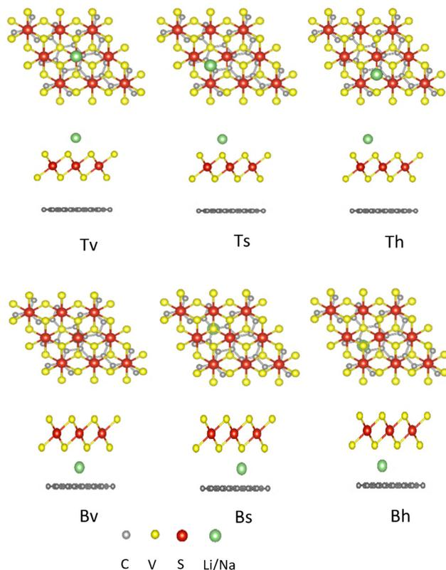
Fig. 6 The adsorption configurations for both Ion/Vs<sub>2</sub>/Gr and Vs<sub>2</sub>/Ion/Gr systems, providing a detailed view of the structural characteristics of each adsorption site.
