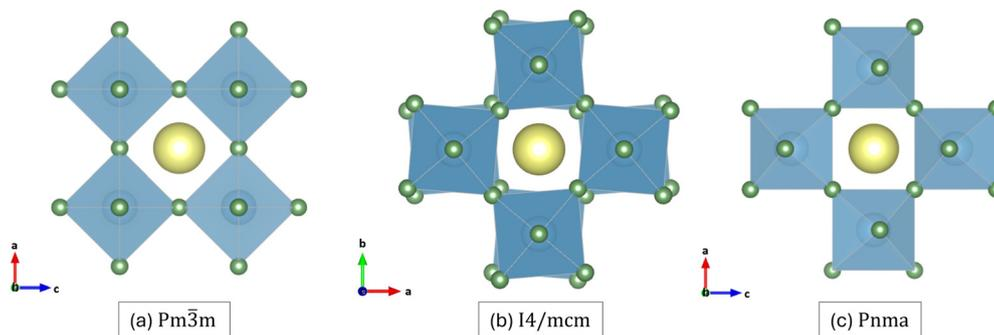
Fig. 1 Optimised structures of SrTiO<sub>3</sub> in the cubic  $Pm\bar{3}m$  (a), tetragonal  $I4/mcm$  (b) and orthorhombic  $Pnma$  phase (c). The  $I4/mcm$  and  $Pnma$  structures are oriented to show the equivalence to the cubic structure.<sup>71</sup> The Sr, Ti and O atoms are shown in yellow, light blue and green respectively. These images were prepared using the VESTA software.<sup>72</sup>
