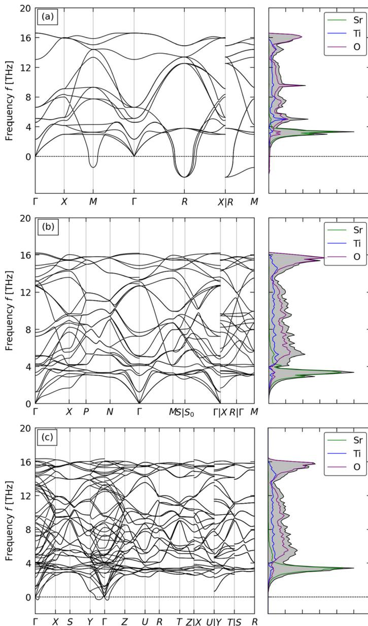
Fig. 2 Calculated phonon dispersion and density of states (DoS) of  $Pm\bar{3}m$  (a),  $I4/mcm$  (b) and  $Pnma$  SrTiO<sub>3</sub> (c). The DoS curves show the total DoS in black/grey with the projections onto the Sr, Ti and O atoms in green, blue and purple respectively.
