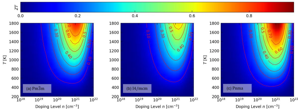
Fig. 8 Predicted scalar-average n-type thermoelectric figure of merit  $zT$  of  $Pm\bar{3}m$  (a),  $I4/mcm$  (b) and  $Pnma$   $SrTiO_3$  (c) as a function of extrinsic carrier concentration (“doping level”)  $n$  and temperature  $T$ .
