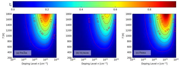
Fig. 8 Predicted scalar-average n-type thermoelectric figure of merit zT of Pm3m (a), I4/mcm (b) and Pnma SrTiO<sub>3</sub> (c) as a function of extrinsic carrier concentration ("doping level") n and temperature T.
