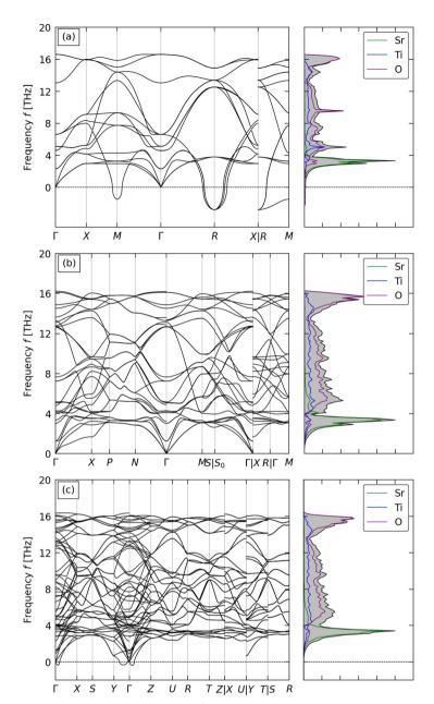
Fig. 2 Calculated phonon dispersion and density of states (DoS) of Pm3m (a), I4/mcm (b) and Pnma SrTiO3 (c). The DoS curves show the total DoS in black/grey with the projections onto the Sr, Ti and O atoms in green, blue and purple respectively.
