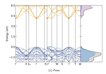
**Fig. 6** Electronic band structure and density of states (DoS) of  $Pm\overline{3}m$  (a), I4/mcm (b) and Pnma SrTiO<sub>3</sub> (c). On each band structure the valence and conduction bands are coloured blue and yellow, respectively, and the valence- and conduction-band minima are marked by green and red circles. On each DoS plot, the total DoS is shown in grey and the projections onto the O 2p and Ti 3d states are shown in blue and pink, respectively.
