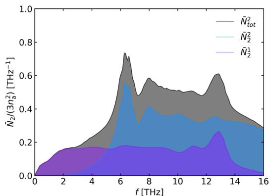
**Fig. 4** Average scattering phase space function  $\tilde{N}_2$  defined in eqn (25) for the *Pm3m* phase of SrTiO<sub>3</sub> at  $T = 1000$  K. The separate phase spaces for collision and decay processes ( $\tilde{N}_2^1/\tilde{N}_2^2$ ) are shown in blue and purple, respectively, and the total phase space is shown in grey.
