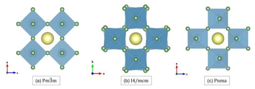
Fig. 1 Optimised structures of SrTiO<sub>3</sub> in the cubic  $Pm\bar{3}m$  (a), tetragonal I4/mcm (b) and orthorhombic Pnma phase (c). The I4/mcm and Pnma structures are oriented to show the equivalence to the cubic structure. The Sr, Ti and O atoms are shown in yellow, light blue and green respectively. These images were prepared using the VESTA software.<sup>72</sup>
