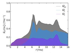
Fig. 4 Average scattering phase space function  $\bar{N}_2$  defined in eqn (25) for the  $Pm\bar{3}m$  phase of  $SrTiO_3$  at T=1000 K. The separate phase spaces for collision and decay processes  $(\bar{N}_2^{(1)}/\bar{N}_2^{(2)})$  are shown in blue and purple, respectively, and the total phase space is shown in grey
