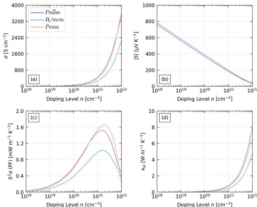
Fig. 7 Predicted scalar-average electrical properties of n-type  $Pm\bar{3}m$ ,  $I4/mcm$  and  $Pnma$  SrTiO<sub>3</sub> as a function of extrinsic carrier concentration  $n$  (“doping level”) at a fixed temperature  $T = 1000$  K: (a) electrical conductivity  $\sigma$ , (b) absolute Seebeck coefficient  $|S|$ , (c) power factor  $S^2\sigma$  (PF), and (d) electronic thermal conductivity  $\kappa_{el}$ .
