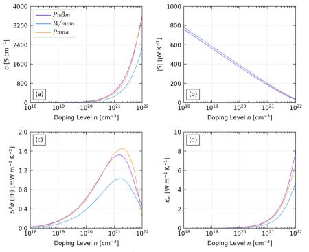
Fig. 7 Predicted scalar-average electrical properties of n-type Pm3m, I4/mcm and Pnma SrTiO<sub>3</sub> as a function of extrinsic carrier concentration n ("doping level") at a fixed temperature T = 1000 K: (a) electrical conductivity  $\sigma$ , (b) absolute Seebeck coefficient |S|, (c) power factor  $S^2\sigma$  (PF), and (d) electronic thermal conductivity  $\kappa_{\rm el}$
