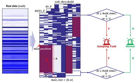
Fig. 9 Flow of the threshold-based detection algorithm
