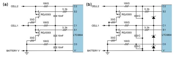
Fig. 2 Sampling board hardware circuit topology: (a) differential filter circuit and (b) ground filter circuit.
