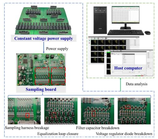
Fig. 3 Test bench of sampling fault injection.
