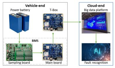
Fig. 1 Vehicle-end to cloud-end battery data transfer flow.
