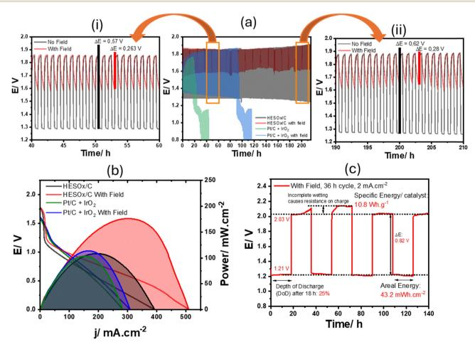
Fig. 4 (a) Discharge profiles of the standards and HESOx/C (1 h cycle, 0.5 mA cm<sup>-2</sup>). Zoomed-in portions of (a) at (i) 50 h and (ii) 200 h. (b) Power profiles of the standard 20% Pt/C + IrO2 cathode and the 20% HESOx/C cathode, with and without an applied field. (c) Deep discharge profile (36 h cycle, 2 mA cm<sup>-2</sup>) of HESOx/C. All data acquired under air.
