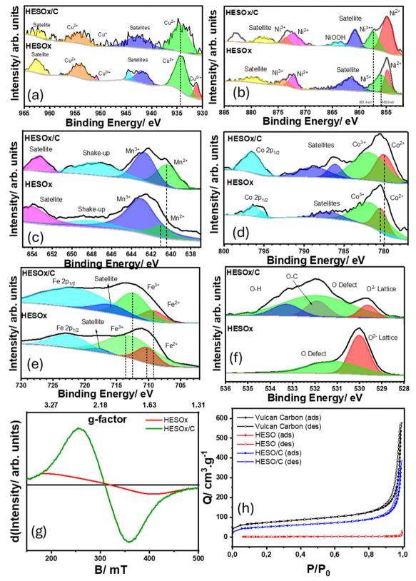
Fig. 3 (a)-(e) shows the deconvoluted 2P XPS spectra of the five metals in both HESOx and HESOx/C. (f) shows the oxygen 1S XPS spectra (g) EPR spectra of HESOx and HESOx/C. (h) N<sub>2</sub> absorption-desorption curves.
