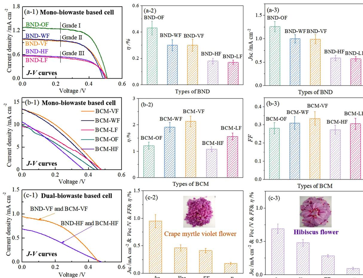
Fig. 2  $J$ - $V$  curves and photovoltaic parameters of renewable-flower-based DSSCs with various modes. (a) Mono-biowaste-based cells using a BND dye and Pt electrode; (b) mono-biowaste-based cells using N719 dye and a BCM electrode; (c) dual-biowaste-based cells using a BND dye and BCM electrode.
