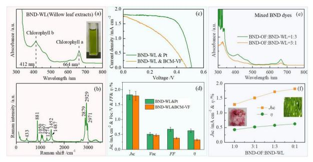
Fig. 8 (a) and (b) UV-Vis and FT-Raman spectra of BND-WL solution. (c) and (d) J-V curves and photovoltaic parameters of DSSCs using various dyes and counter electrodes. (e) UV-Vis spectra of the mixed solution of BND-OF and BND-WL, and (f) their photovoltaic parameters in DSSCs with a Pt electrode
