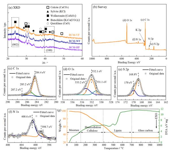
Fig. 7 Structure and surface characteristics of various pyrolyzed flower BCMs. (a) XRD patterns. (b) XPS survey spectrum and high-resolution scans of the (c) C 1s, (d) O 1s, (e) S 2p and (f) N 1s regions of BCM-VF. (g) TGA and DTA curves of the dried crape myrtle violet flower used for BCM-VF preparation.
