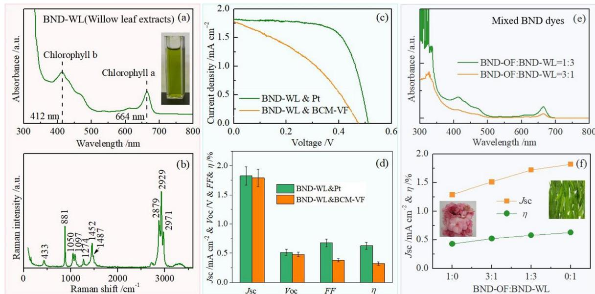
Fig. 8 (a) and (b) UV-Vis and FT-Raman spectra of BND-WL solution. (c) and (d)  $J$ - $V$  curves and photovoltaic parameters of DSSCs using various dyes and counter electrodes. (e) UV-Vis spectra of the mixed solution of BND-OF and BND-WL, and (f) their photovoltaic parameters in DSSCs with a Pt electrode.
