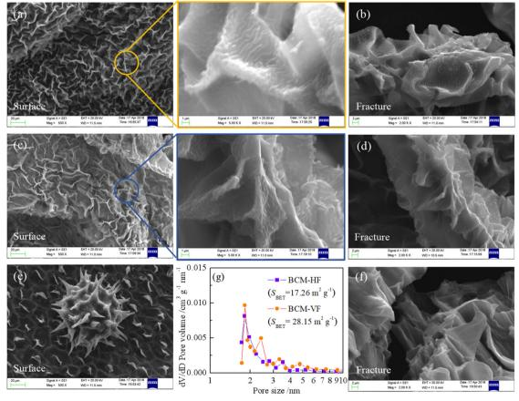
Fig. 5 Morphological and porous characteristics of various pyrolyzed flower BCMs. (a) and (b) SEM images of BCM-VF; (c) and (d) SEM images of BCM-VF WF; (e) and (f) SEM images of BCM-HF; (g) pore size distributions of BCM-VF and BCM-HF.
