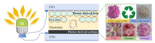
Fig. 1 Schematic of DSSCs consisting of natural anthocyanin dyes and natural carbon counter electrodes derived from renewable flowers.
