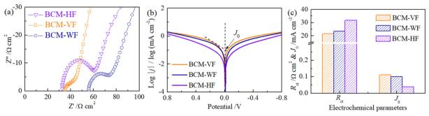
Fig. 3 Electrochemical performances of the various BCM counter electrodes. (a) Nyquist plots; (b) Tafel polarization curves; (c) electrochemical parameters extracted from (a) and (b).
