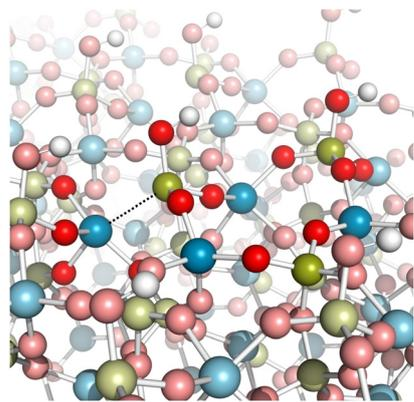
Fig. 2 Structural model of (P-OH)<sub>2</sub>-berlinite with the Al–P dative bond depicted by a dashed line. Al, P, O, and H atoms are represented in blue, green, red, and white, respectively.
