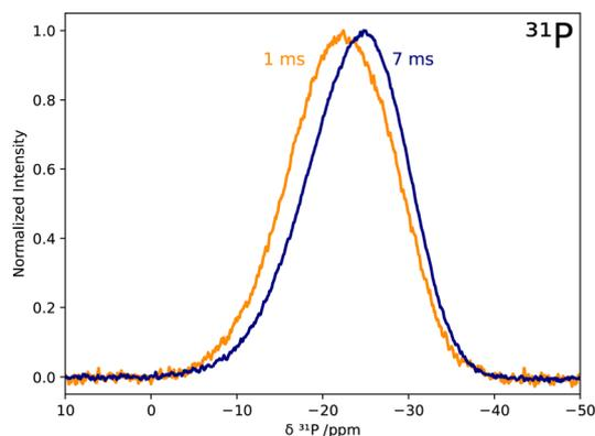
Fig. 6  $^{31}\text{P}\{^1\text{H}\}$  CPMAS NMR spectra of dried  $\text{AlPO}_4$  for a contact time of 1 ms (orange) and of 7 ms (blue) with a MAS spinning rate of 10 kHz. The spectra were normalized to the respective maximum intensity.
