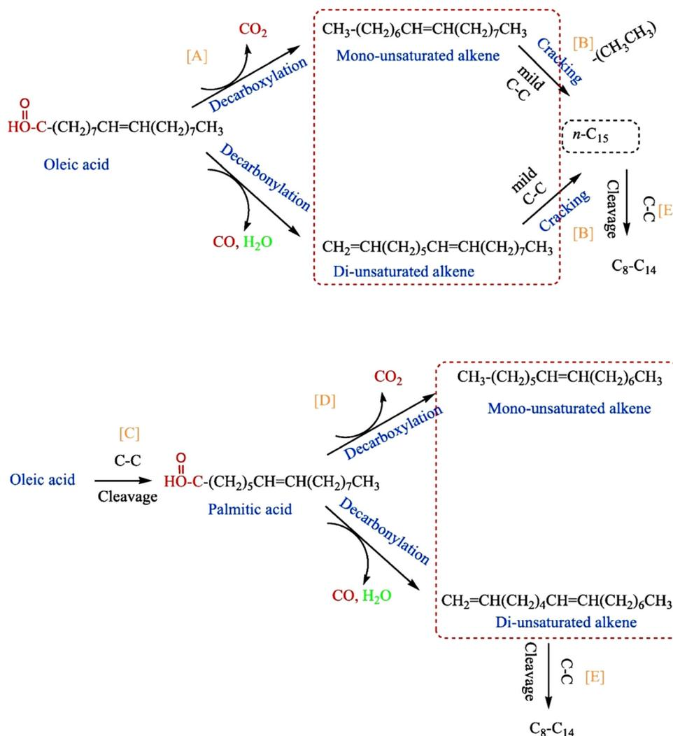
Fig. 3 Proposed deoxygenation reaction pathway for the deoxygenation of WCO to hydrocarbon over CaO–La<sub>2</sub>O<sub>3</sub>/AC catalysts.
