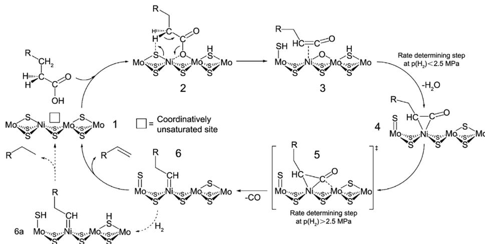
Fig. 5 Hypothesized mechanism for the decarbonylation of fatty acids on Ni-MoS<sub>2</sub>. Reprinted with permission from ref. 276.
