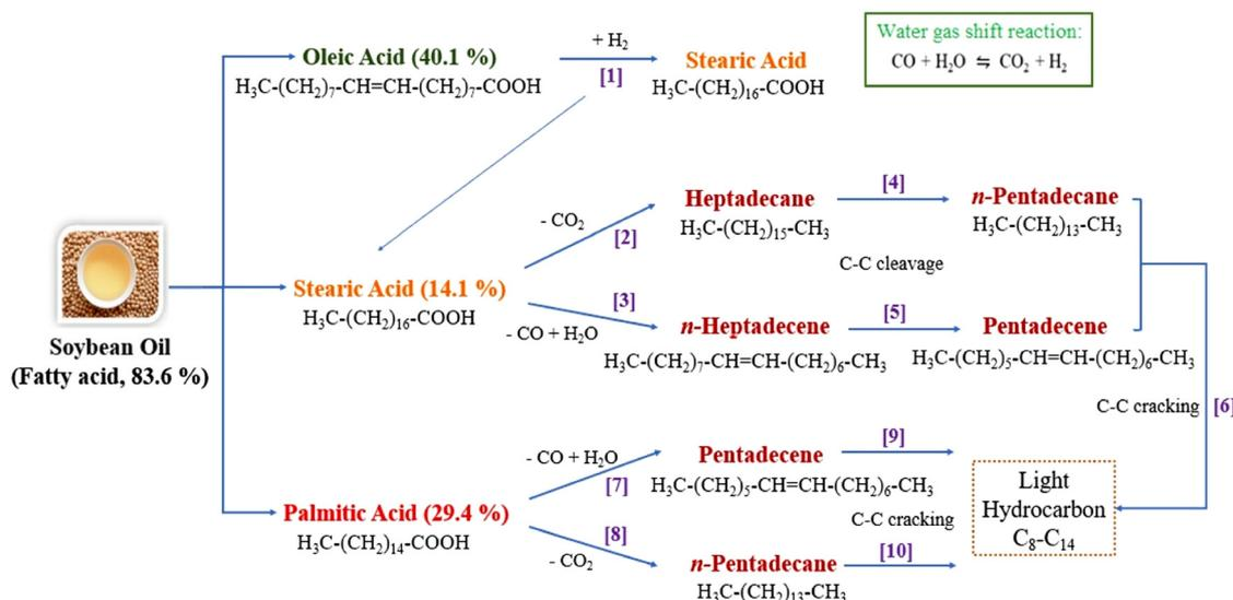
Fig. 4 Proposed catalytic deoxygenation reaction mechanism of soybean oil using a NiO–CD catalyst.<sup>118</sup>
