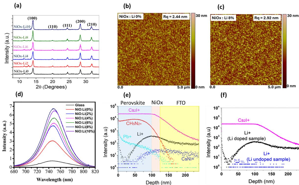
Fig. 2 (a) XRD patterns of perovskite films deposited on different Li-doped NiO<sub>x</sub> films, (b) AFM image of Li-0% NiO<sub>x</sub>, (c) AFM image of Li-8% NiO<sub>x</sub>, (d) steady state PL intensity of perovskite films deposited on different Li-doped NiO<sub>x</sub> films, (e) TOF-SIMS depth profile for the device grown on Li-4% NiO<sub>x</sub>, and (f) comparison of Li concentrations in the TOF-SIMS profile for devices grown on Li-4% and Li-0% NiO<sub>x</sub> films.
