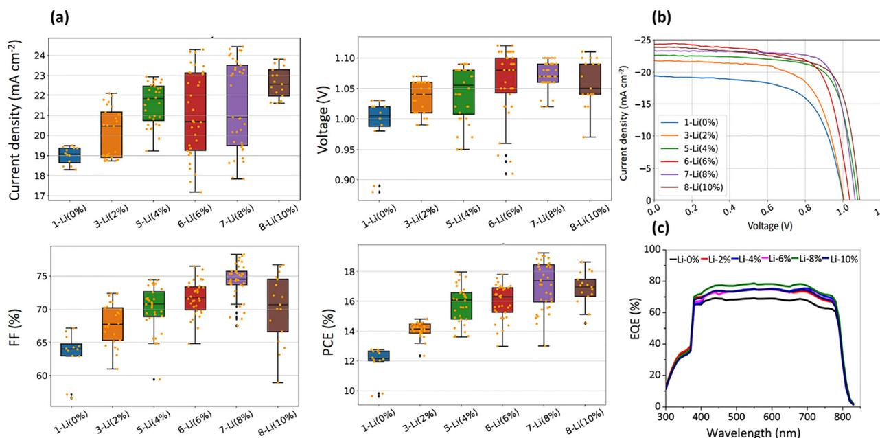
Fig. 4 (a) Device performances of PSCs with different Li-doped NiO<sub>x</sub> HTLs, (b) *J*-*V* curves of the best cells for different Li-doped NiO<sub>x</sub> devices and (c) EQE plot of perovskite solar cells on different Li-doped NiO<sub>x</sub> HTLs.
