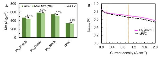
Fig. 6 (A) MAs at 0.9 V before (initial) and after ADT (70k) of Pt<sub>3.7</sub>Mn/KB, Pt<sub>3.9</sub>Co/KB, Pt<sub>3.7</sub>Ni/KB and cPt/C in O<sub>2</sub>-saturated 0.1 M HClO<sub>4</sub>. (B) I-V polarization curves of Pt<sub>3.9</sub>Co/KB and cPt/C measured at 80 °C, 75% RH, H<sub>2</sub>/Air 50 kPa-G
