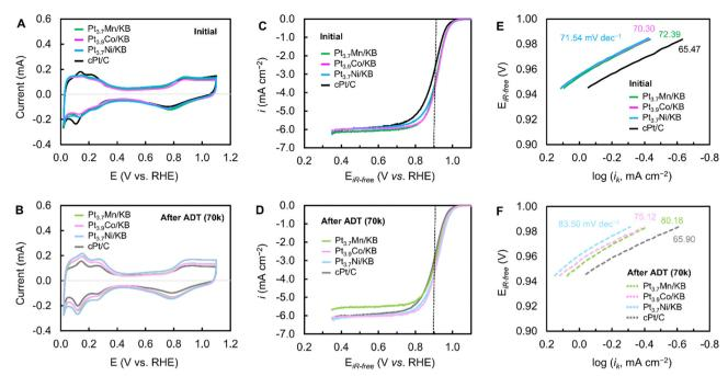
Fig. 5 The CVs (A) and (B), LSVs (C) and (D) and Tafel slopes (E) and (F) of Pt<sub>3.7</sub>Mn/KB, Pt<sub>3.9</sub>Co/KB and Pt<sub>3.7</sub>Ni/KB along with cPt/C before (A), (C) and (E) and after (B), (D) and (F) ADT (70k). CVs (at 0 rpm) and LSVs (at 1600 rpm) were measured in the N2- and O2-saturated 0.1 M HClO4 electrolyte, respectively. The Tafel slopes were estimated from the kinetic currents at 0.945-0.983 V.
