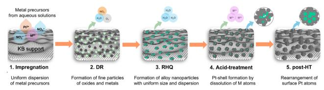
Fig. 1 A general scheme for the ASI-RHQ preparation method of the core-shell structured alloy catalysts.
