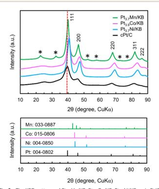
Fig. 2 The XRD patterns of Pt<sub>3.7</sub>Mn/KB, Pt<sub>3.9</sub>Co/KB, Pt<sub>3.7</sub>Ni/KB and cPt/C. Asterisks indicate the ordered phase of Pt<sub>3.7</sub>Mn/KB. The reference diffraction peak positions of bulk Mn, Co, Ni and Pt are also shown below.
