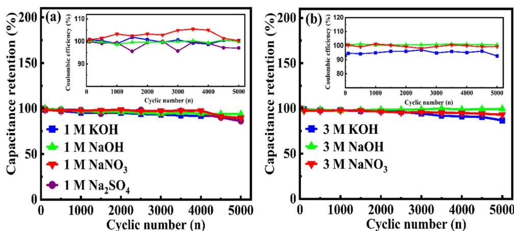
Fig. 18 Cyclic performance of  $\text{Mn}_2\text{O}_3\text{-9}$  in (a) 1 M and (b) 3 M concentrations of electrolytes. The inset displays the Coulombic efficiency (CE) measured at  $10 \text{ A g}^{-1}$  current density.
