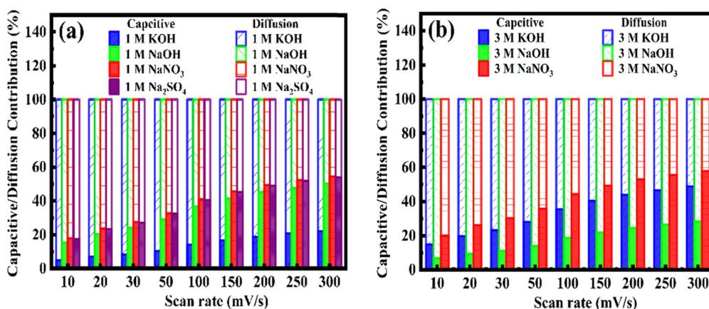
Fig. 12 Percentage capacitive and diffusion contribution to the total charge storage in the  $\text{Mn}_2\text{O}_3\text{-9}$  mM urea sample measured in (a) 1 M and (b) 3 M electrolyte concentrations at different scan rates.
