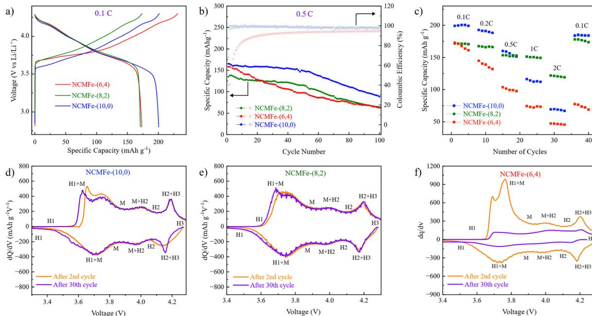
Fig. 7 Comparison of electrochemical performance of NCMFe-(10,0), NCMFe-(8,2) and NCMFe-(6,4), in terms of (a) charge–discharge at 0.1C; (b) cycling performance at 0.5C, and (c) rate capability. The differential capacity ( $dQ/dV$ ) profiles of (d) NCMFe-(10,0), (e) NCMFe-(8,2) and (f) NCMFe-(6,4).
