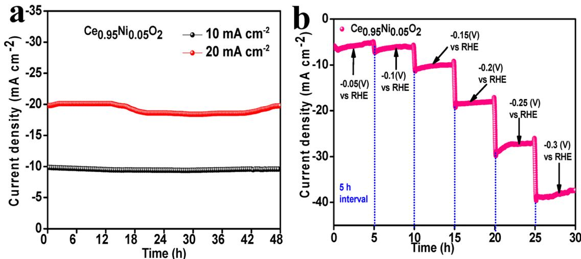
Fig. 6 (a) Stability studies with Ce<sub>0.95</sub>Ni<sub>0.05</sub>O<sub>2</sub> at 10 and 20 mA cm<sup>-2</sup> and (b) stepwise CA study of Ce<sub>0.95</sub>Ni<sub>0.05</sub>O<sub>2</sub>.
