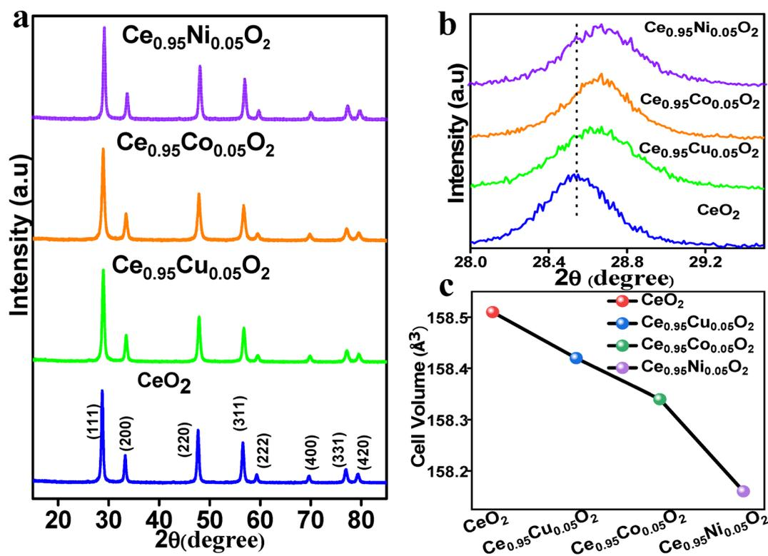
Fig. 2 (a) XRD patterns, (b) zoomed in version, (c) the refined cell volume of  $\text{CeO}_2$  and doped  $\text{Ce}_{0.95}\text{Co}_{0.05}\text{O}_2$ ,  $\text{Ce}_{0.95}\text{Ni}_{0.05}\text{O}_2$ , and  $\text{Ce}_{0.95}\text{Cu}_{0.05}\text{O}_2$ .
