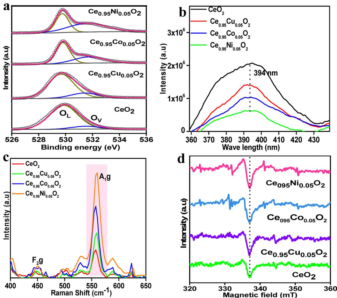
Fig. 4 (a) O1s core level XPS spectra; (b) PL; (c) Raman and (d) EPR spectra of CeO<sub>2</sub> and doped Ce<sub>0.95</sub>Co<sub>0.05</sub>O<sub>2</sub>, Ce<sub>0.95</sub>Ni<sub>0.05</sub>O<sub>2</sub> and Ce<sub>0.95</sub>Cu<sub>0.05</sub>O<sub>2</sub>.
