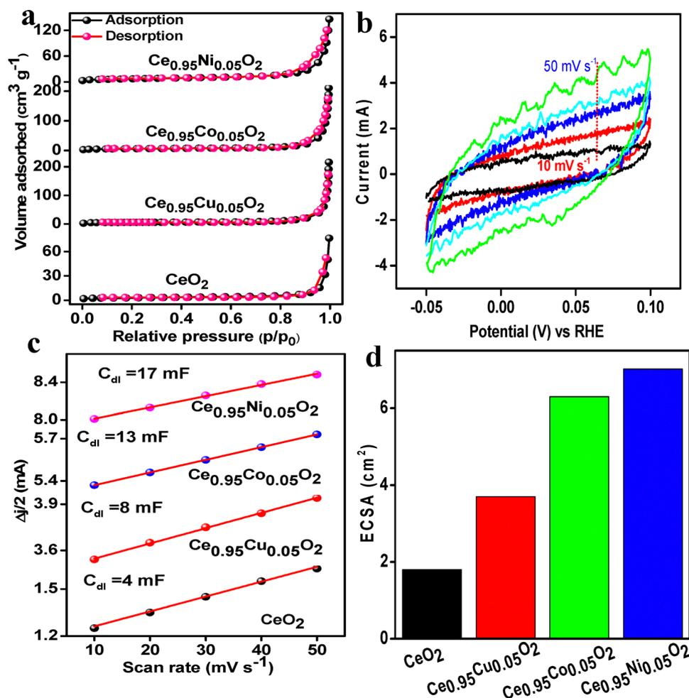
Fig. 3 (a)  $\text{N}_2$  adsorption-desorption isotherms of the synthesized catalysts; (b) CV curves of  $\text{Ce}_{0.95}\text{Ni}_{0.05}\text{O}_2$  in the non-faradaic region (-0.05 to 0.1 V vs. RHE) at scan rates of 10, 20, 30, 40, 50  $\text{mV s}^{-1}$ ; (c) linear regression between the current density differences in the 0.02 V potential window of CV vs. scan rate and (d) ECSA of all four catalysts.
