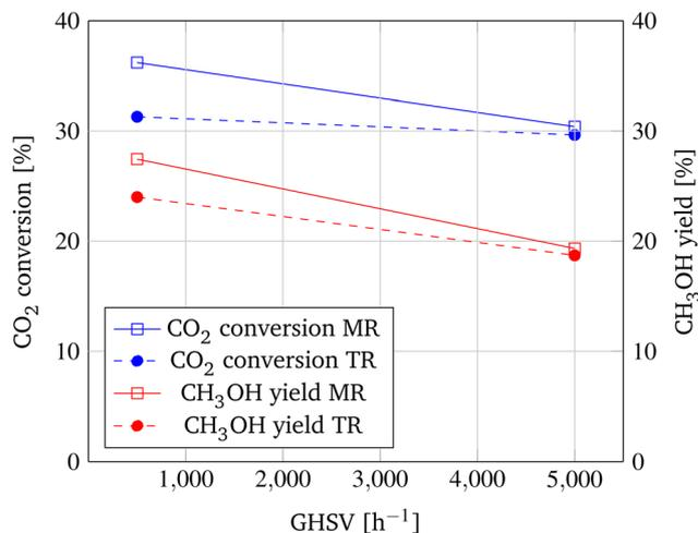
Fig. 9 Main effect of GHSV on CO<sub>2</sub> conversion and CH<sub>3</sub>OH yield at 100 bar and 250 °C.
