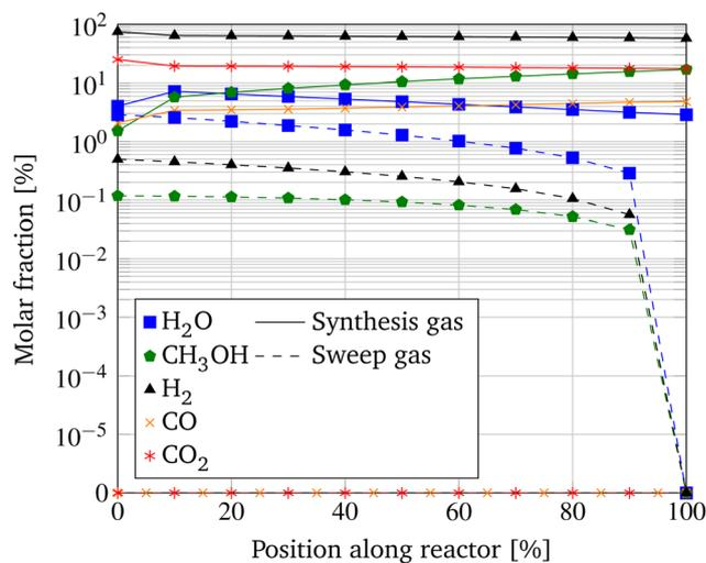
Fig. 12 Molar fractions along the length of the MR with best case parameters (GHSV = 500  $\text{h}^{-1}$ ,  $S/F$  ratio = 10,  $O_M/V_R$  ratio = 133.3  $\text{m}^{-1}$ ) at a pressure of 100 bar and a temperature of 250 °C.
