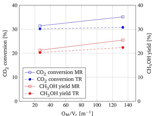
Fig. 10 Main effect of  $O_M/V_r$  ratio on CO<sub>2</sub> conversion and CH<sub>3</sub>OH yield at 100 bar and 250 °C.
