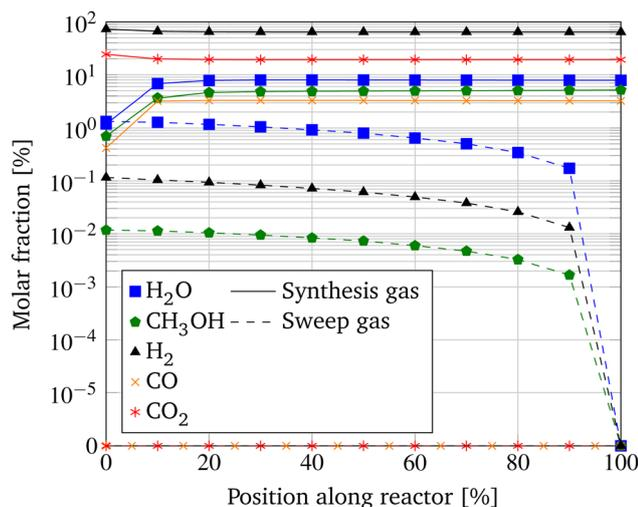
Fig. 6 Molar fractions along the length of the MR with base case parameters at a pressure of 100 bar and a temperature of 250 °C.
