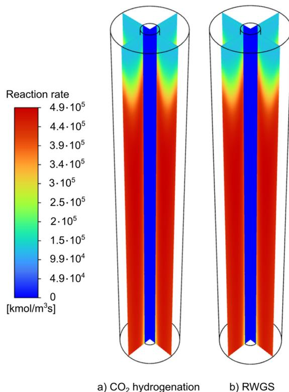
Fig. 7 Profiles of the (a) CO<sub>2</sub> hydrogenation and (b) RWGS reaction rates along the length of the MR with base case parameters at a pressure of 100 bar and a temperature of 250 °C.
