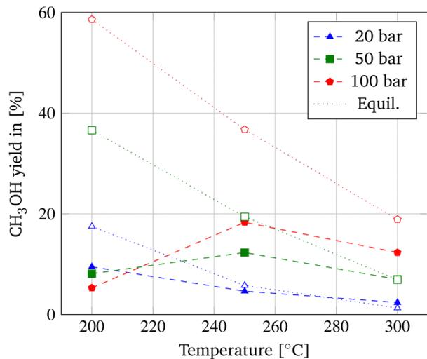
Fig. 4 Pressure and temperature dependency of CH<sub>3</sub>OH yield of the MR (dashed lines) and equilibrium CH<sub>3</sub>OH yields from ref. 9 (dotted lines).
