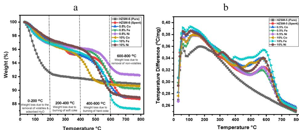
Fig. 14 present the TGA (a) and DTA (b) of spent metal-doped HZSM-5 catalysts. Reproduced from ref. 87 with permission from Elsevier, copyright 2024. The data indicate that increasing metal loading from 0.5 to 10 wt% correlates with higher mass loss, primarily attributed to enhanced coke deposition on the HZSM-5 surface.
