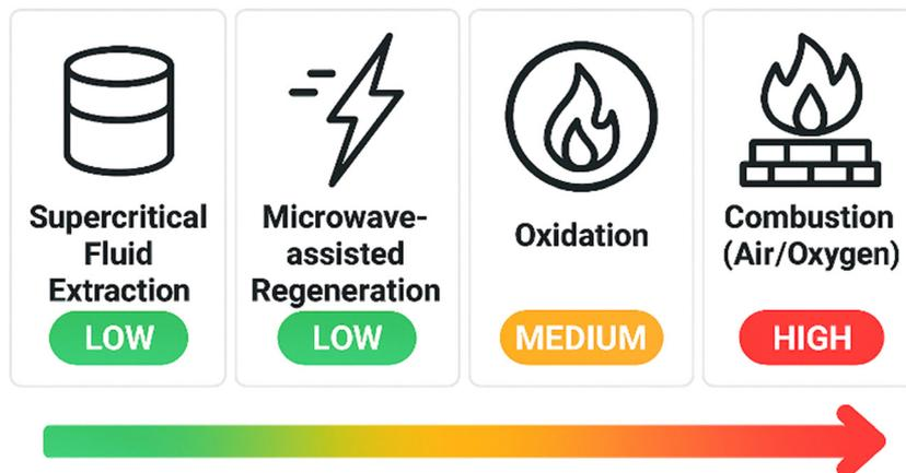
Fig. 27 Severity of emissions from different regeneration methods.
