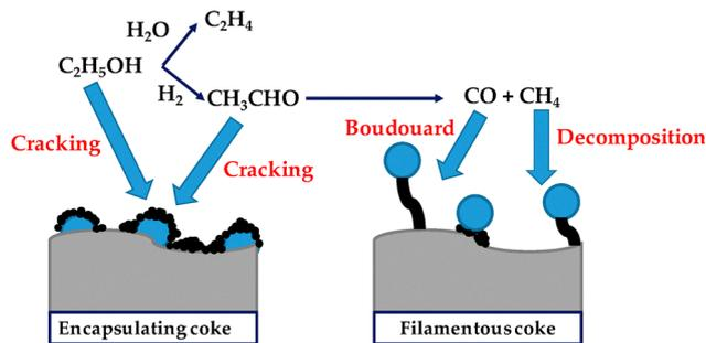
Fig. 13 Formation mechanism and characteristics of coke deposits on Ni/La<sub>2</sub>O<sub>3</sub>- $\alpha$ -Al<sub>2</sub>O<sub>3</sub> catalyst. Reproduced from ref. 78 with permission from MDPI, copyright 2020.
