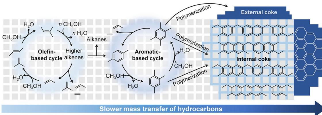
Fig. 11 Proposed pathways for reaction progression and coke formation mechanism during the methanol-to-hydrocarbons (MTH) conversion process. Reproduced from ref. 52 with permission from Elsevier, copyright 2019.
