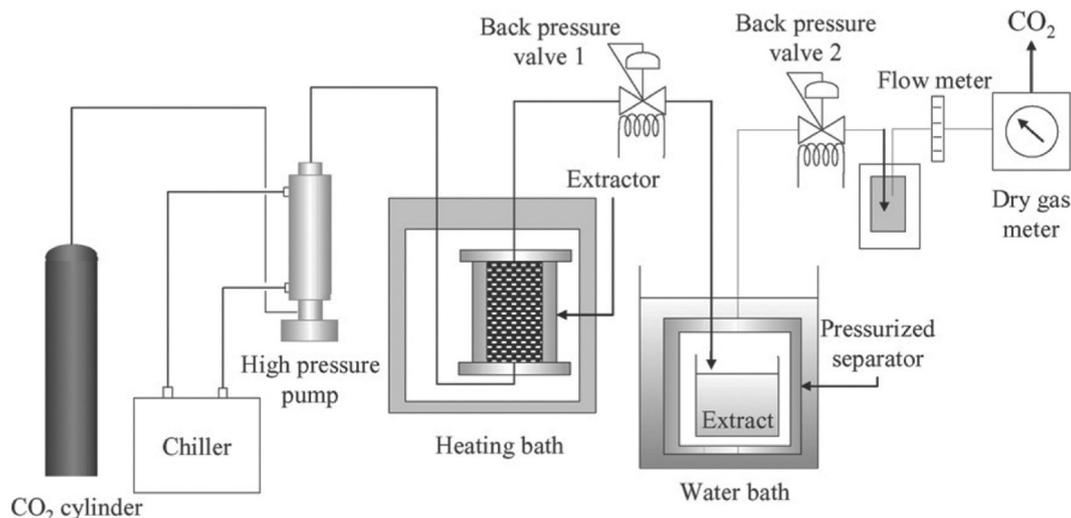
Fig. 20 Schematic diagram of supercritical fluid extraction (SFE) set-up. Reproduced from ref. 166 with permission from Elsevier, copyright 2006.
