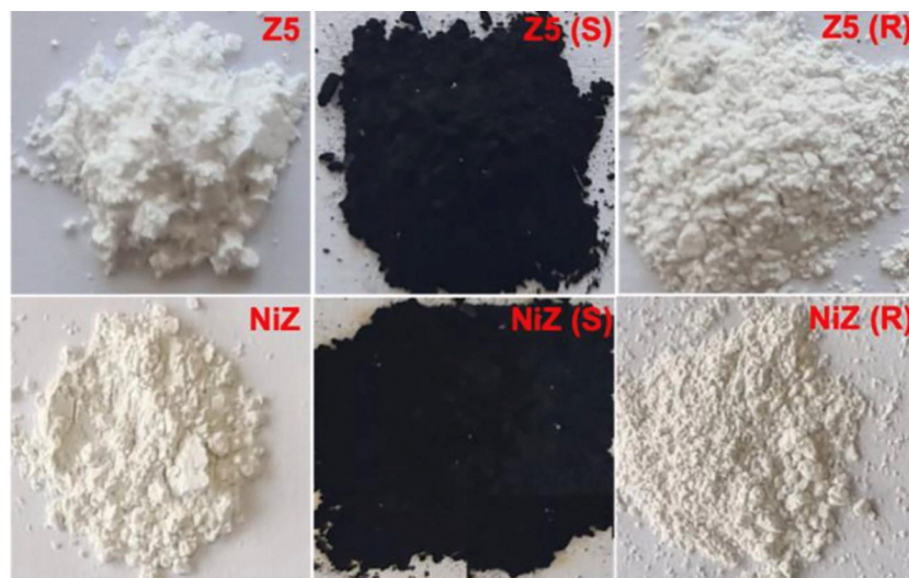
Fig. 18 Images of the fresh catalyst (Z5 and NiZ) spent (Z5 (S) and NiZ (S)) and regenerated (Z5 (R) and NiZ (R)) zeolite catalysts. Reproduced from ref. 114 with permission from Elsevier, copyright 2024.
