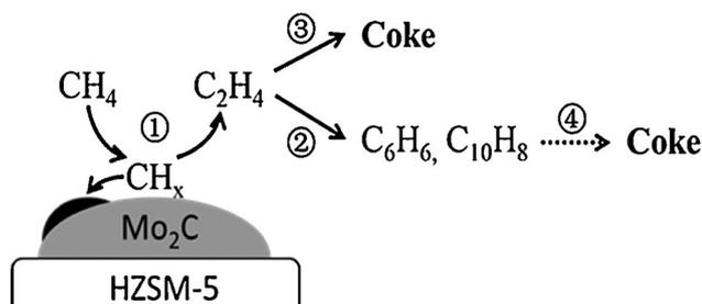
Fig. 12 Schematic diagram of coking pathways during CH<sub>4</sub> conversion over Mo<sub>2</sub>C/HZSM-5 catalyst. Reproduced from ref. 68 with permission from Elsevier, copyright 2014.
