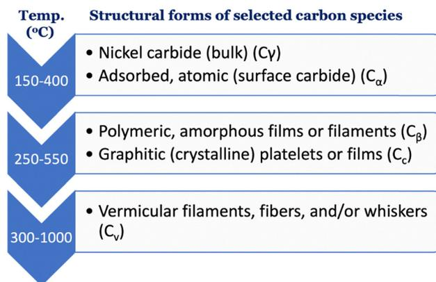
**Fig. 6** Structural forms of different kinds of carbon species generated by CO decomposition on Ni catalysts. Carbon classifications: C<sub>γ</sub>: metal carbide, C<sub>α</sub>: adsorbed atomic carbon, C<sub>β</sub>: polymeric carbon film, C<sub>c</sub>: amorphous and graphitic carbon, C<sub>v</sub>: vermicular carbon. Modified from ref. 5.
