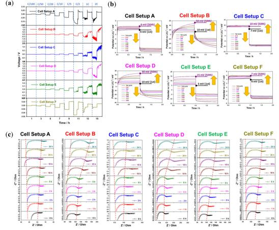
Fig. 4 (a) Critical current densities, (b) plating and stripping process at current densities of C/20, and (c) Nyquist plots at various storage times for 24 h of cell setup from Fig. 2 at various current densities.
