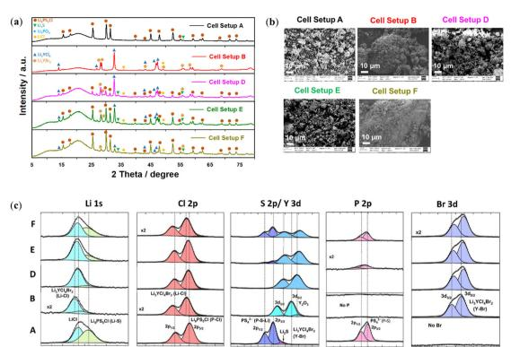
Fig. 3 (a) The XRD patterns, (b) the SEM images and (c) XPS analysis of the samples A, B, D, E and F. All the spectra were calibrated by adjusting the C 1s (C-C/C-H) peak at 284.8 eV.
