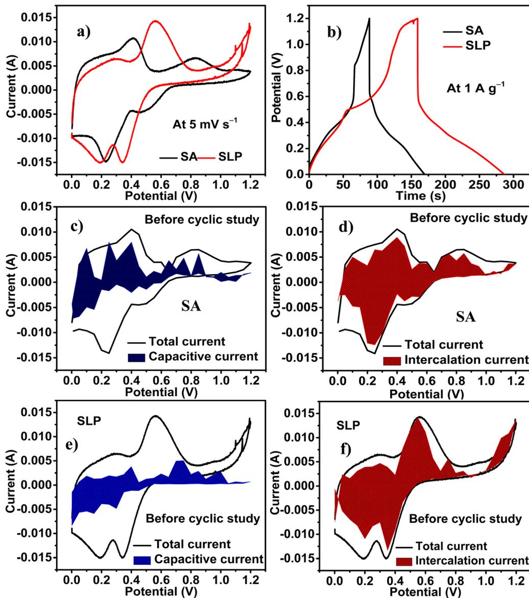
Fig. 4 (a) CV plots at  $5 \text{ mV s}^{-1}$ , (b) charge and discharge (CD) plots at  $1 \text{ A g}^{-1}$  of PZnSn ITPO SA and SLP, (c) and (d) capacitive and intercalation current offered by PZnSn ITPO SA at  $5 \text{ mV s}^{-1}$ , (e) and (f) capacitive and intercalation current offered by PZnSn ITPO SLP at  $5 \text{ mV s}^{-1}$ .
