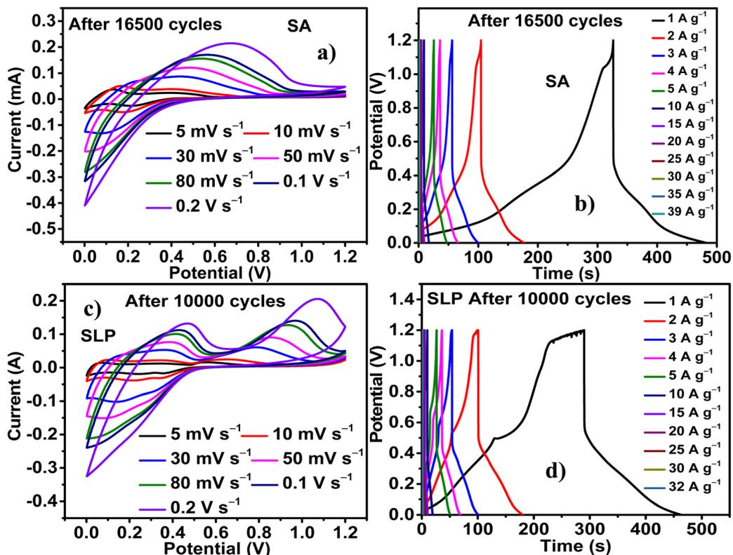
Fig. 8 (a) CV plots at different scan rates and (b) CD plots at different current densities of PZnSn after 16 500 cycles ITPO SA, (c) CV plots at different scan rates, and (d) CD plots at different current densities of PZnSn after 10 000 cycles ITPO SLP.
