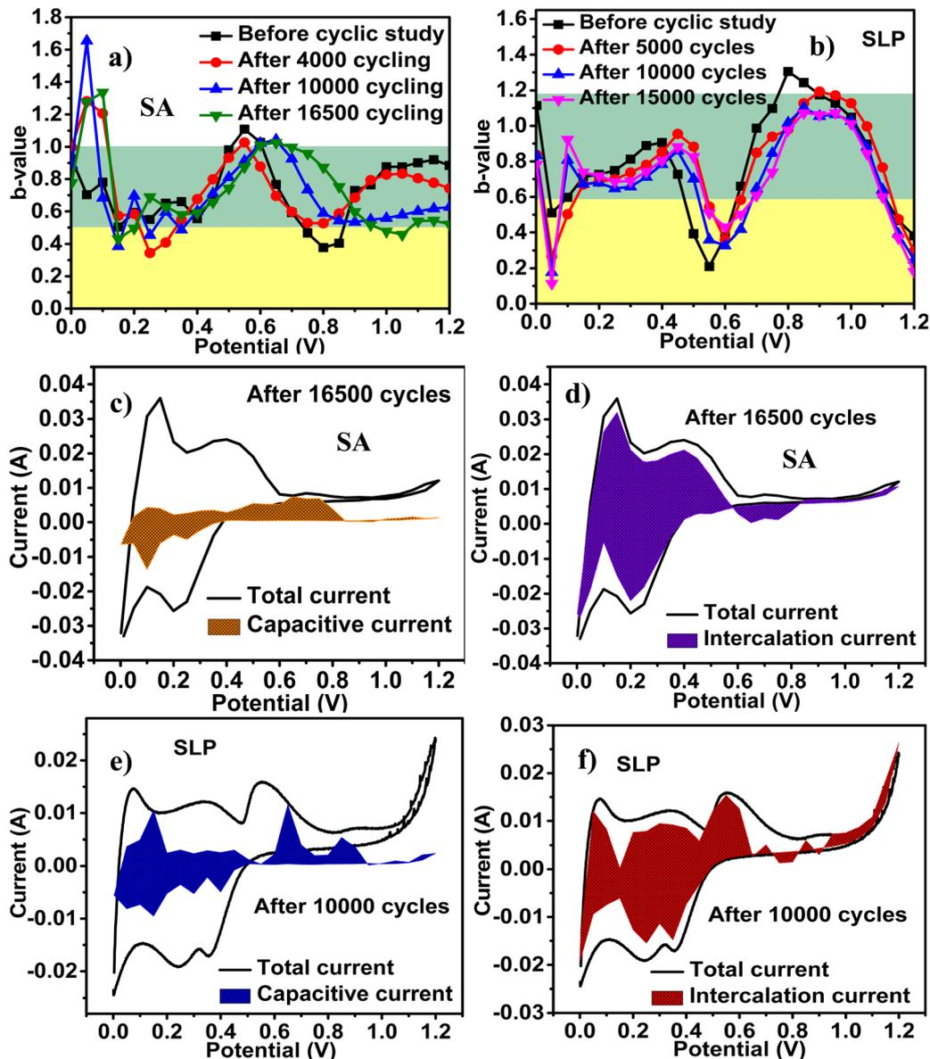
Fig. 6 Plots of  $b$ -value vs. potential of PZnSn ITPO (a) SA & (b) SLP after DNC. The deconvolution of the CV curve of PZnSn ITPO SA was obtained after 16 500 cycles, providing (c) capacitive current and (d) intercalation current. The deconvolution of the CV curve of PZnSn ITPO SLP was obtained after 10 000 cycles, providing (e) capacitive current and (f) intercalation current.
