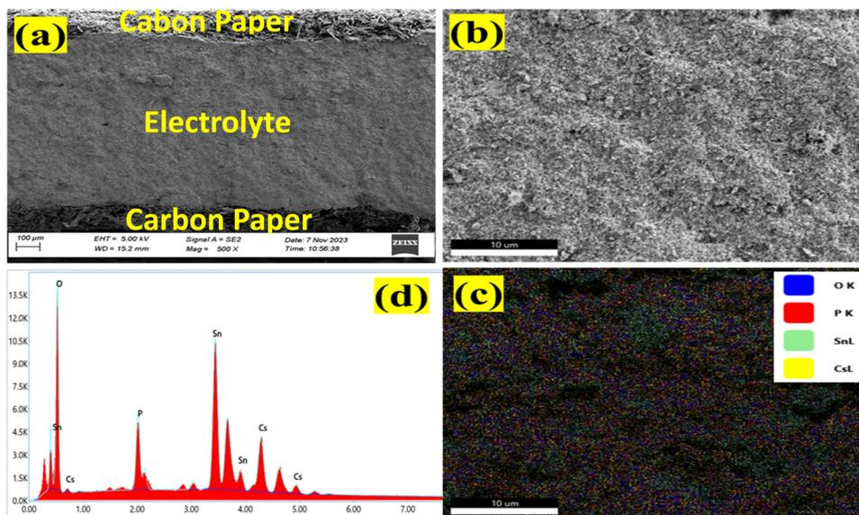
Fig. 2 (a) The cross-sectional view of CDP/SnO<sub>2</sub> sandwiched between carbon paper. (b) and (c) EDX of the CDP/SnO<sub>2</sub> composite electrolyte. (d) The elemental mapping of the CDP/SnO<sub>2</sub> composite electrolyte.
