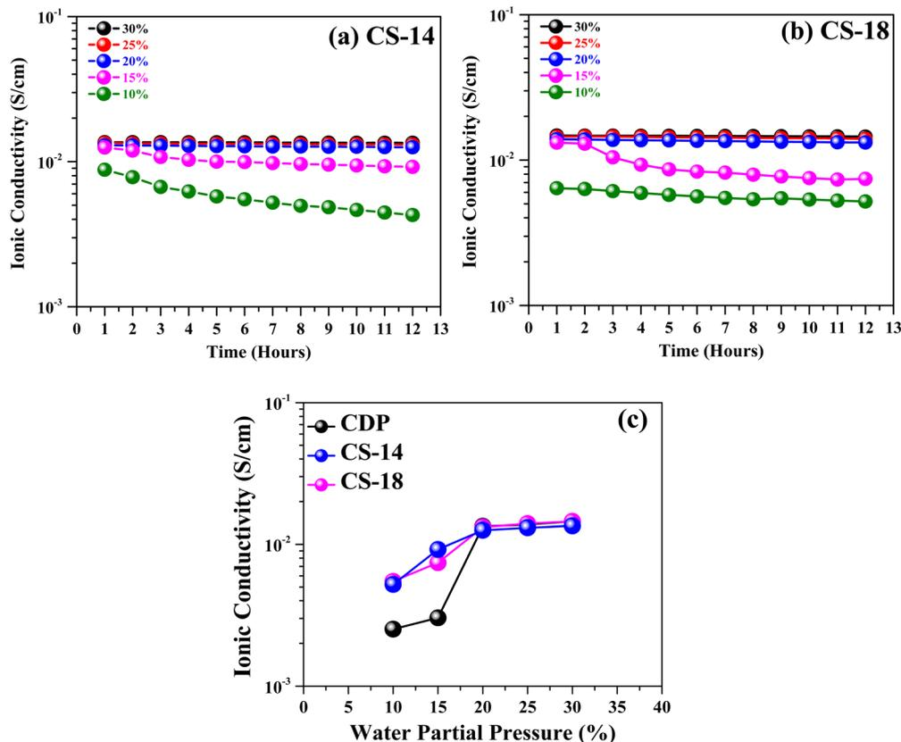
Fig. 8 Time-dependent conductivity of composite electrolytes at 250 °C in wet  $H_2$  atmosphere with 30 mL  $min^{-1}$  flow rate on both sides at different water partial pressures: (a) CS-14 and (b) CS-18. (c) Comparative conductivities of CDP, CS-14, and CS-18 at different partial pressures.
