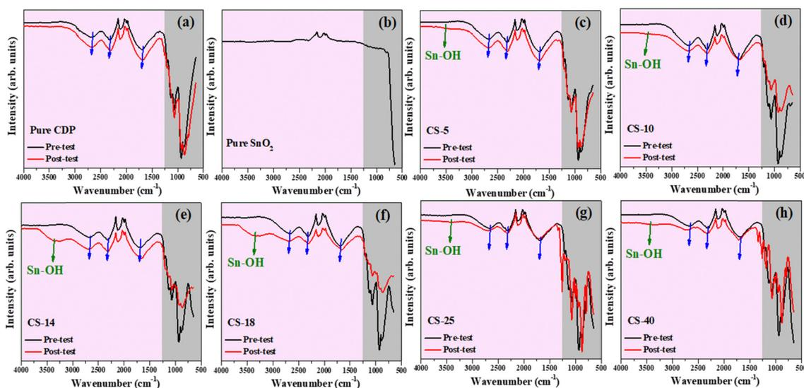
Fig. 9 (a)–(h) FTIR spectra for pure and composite CDP/ $SnO_2$  electrolytes.
