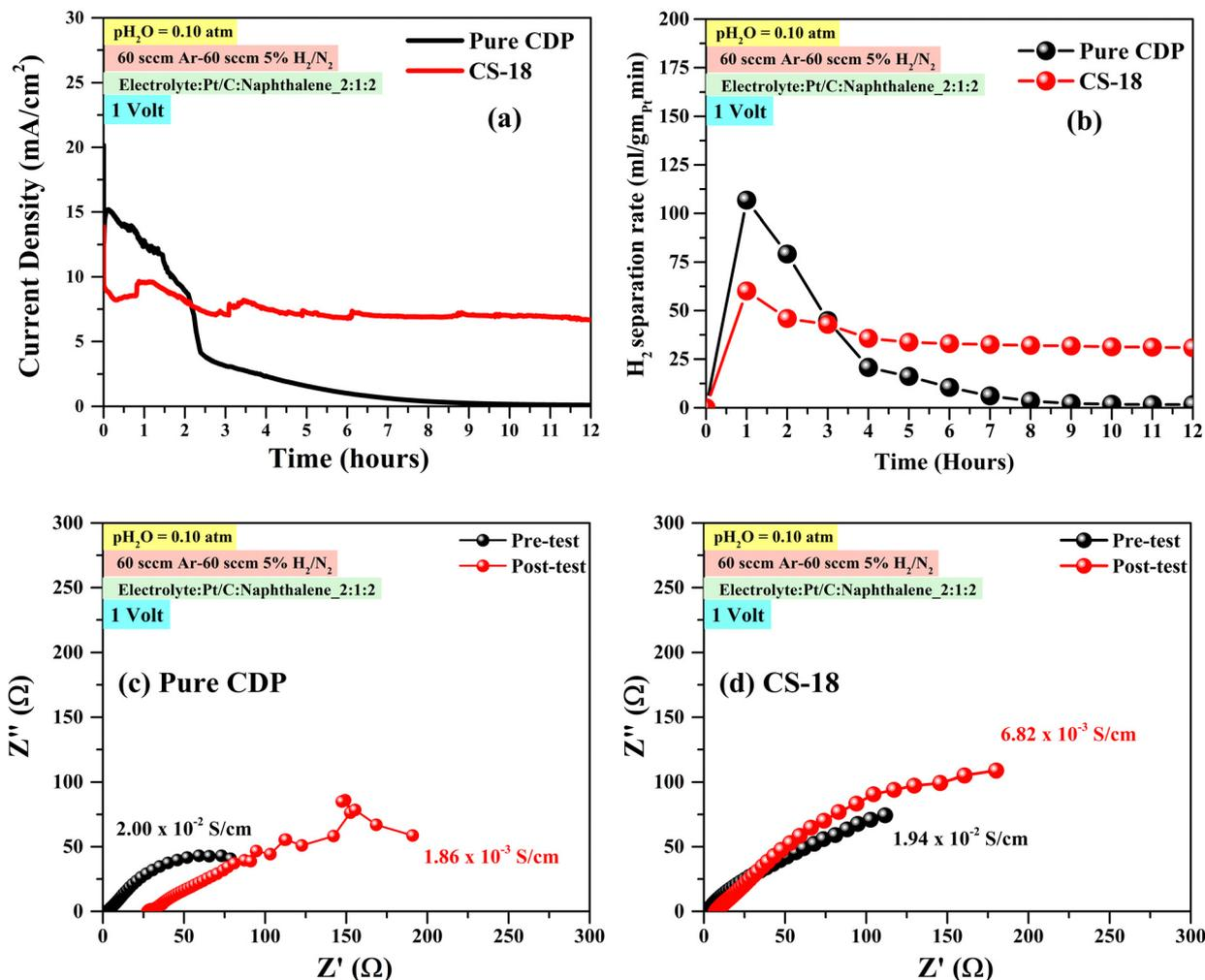
Fig. 10 (a) Chronoamperometry at 1 volt, 250 °C and  $p_{\text{H}_2\text{O}} = 0.10$  for CS-18 and CDP membrane. (b) The rate of  $\text{H}_2$  pumped at 1 volt. (c) and (d) EIS spectra of the pre- and post-test samples.
