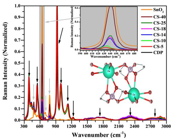
Fig. 3 Raman spectra of the CDP/SnO<sub>2</sub> composite electrolyte; the black arrow indicates shifts corresponding to CDP and the grey arrow indicates shifts related to SnO<sub>2</sub>. The representative crystal structure is extracted from VESTA software.
