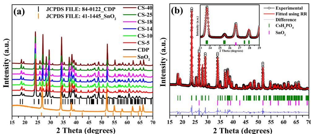
Fig. 1 (a) X-ray diffraction patterns of pure CDP and composite CDP/SnO<sub>2</sub> electrolyte. (b) Rietveld refinement patterns of CS-25 (75CDP : 25SnO<sub>2</sub>).
