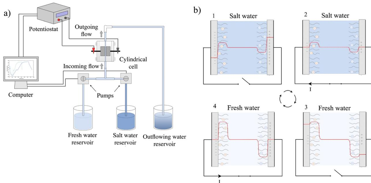
**Fig. 2** (a) Scheme of the experimental setup required for the salinity exchange energy extraction process. (b) Potential profile during energy extraction cycle divided in four stages: (1) salty water, open circuit; (2) salty water; closed circuit, applied positive current value for charge transfer; (3) fresh water, open circuit; (4) fresh water, closed circuit, applied current value of opposite sign.
