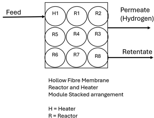
Fig. 3  $3 \times 3$  simultaneous heating and cracking HFMR module.
