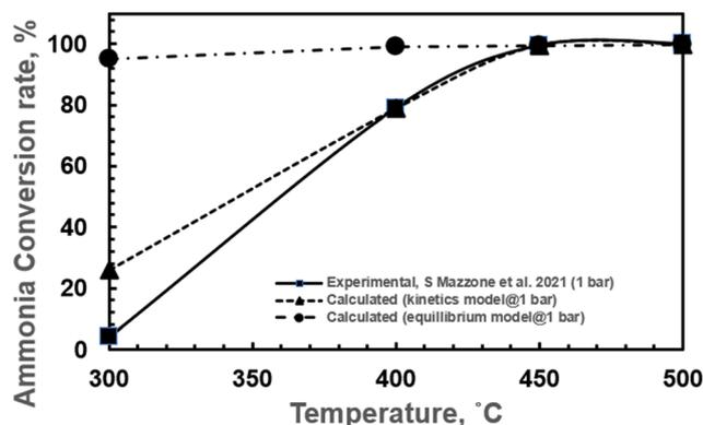
Fig. 6 Conversion vs. temperature for experimental data (S. Mazzone et al. (2021)),<sup>32</sup> equilibrium model and kinetic model across temperatures ranging from 300 °C to 500 °C and pressures.
