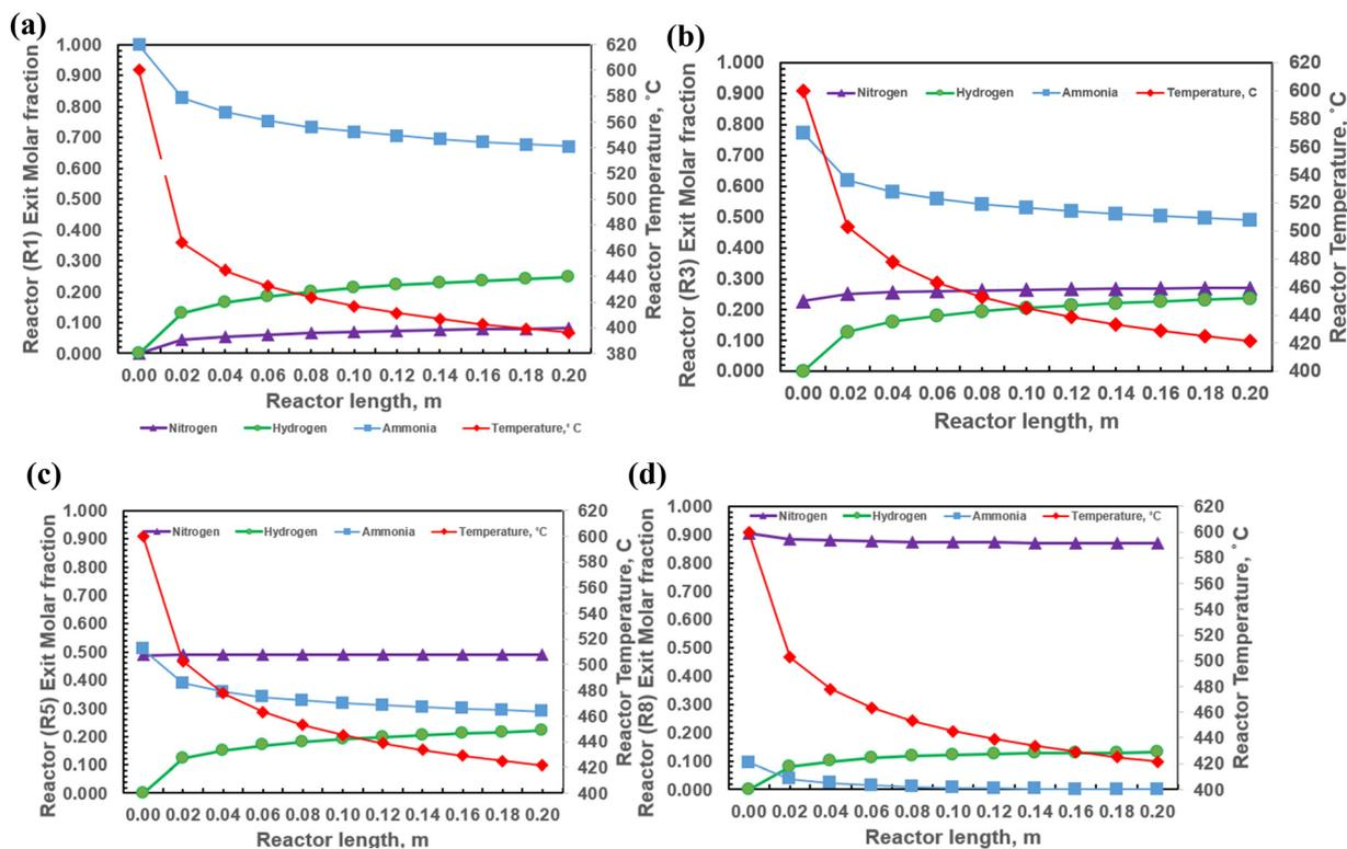
Fig. 9 (a)  $4 \times 4$  intermediate heating and cracking HFMR module (reactor R1 performance profile). (b)  $4 \times 4$  intermediate heating and cracking HFMR module (reactor R3 performance profile). (c)  $4 \times 4$  intermediate heating and cracking HFMR module (reactor R5 performance profile). (d)  $4 \times 4$  intermediate heating and cracking HFMR module (reactor R8 performance profile).
