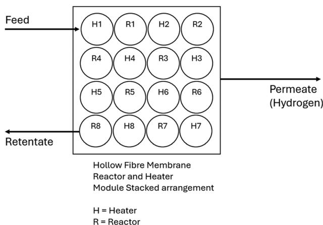
Fig. 4  $4 \times 4$  intermediate heating and cracking HFMR module.
