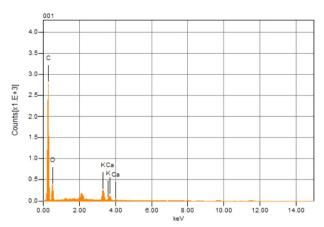
Fig. 3 EDX analysis of Citrus limetta waste
