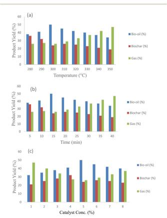
Fig. 6 Pyrolysis of Citrus limetta loaded with zeolite  $\beta$ , ammonium. (a) Temperature optimization, (b) time optimization, and (c) catalyst optimization.
