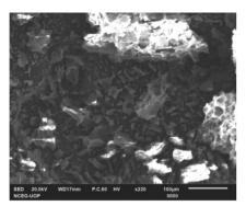
Fig. 2 SEM image of Citrus limetta waste
