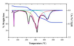
Fig. 4 TG/DTG analysis of Citrus limetta waste in the presence of zeolite  $\beta$ , ammonium at a heating rate of 15 °C min<sup>-1</sup>.
