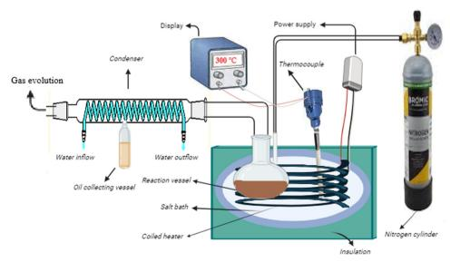
Fig. 1 Schematic of the pyrolysis setup
