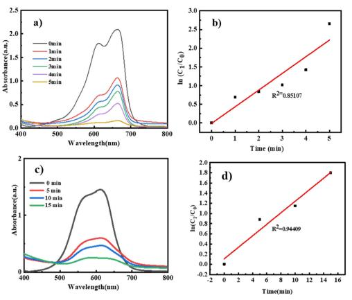
(a) and (c) UV-Vis spectra of MB and VB degradation using VC-5 and (b) and (d) adsorption kinetics of MB and VB dye using VC-5.
