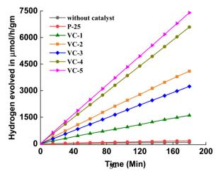
Fig. 8 Photocatalytic hydrogen generation via H<sub>2</sub>O splitting of a system without catalyst, P25, VC-1 to VC-5.
