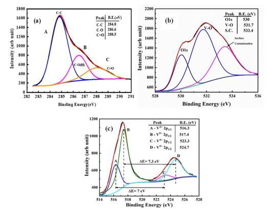
Fig. 5 XPS spectra of VC-5: (a) C 1s, (b) O 1s and (c) V 2p.
