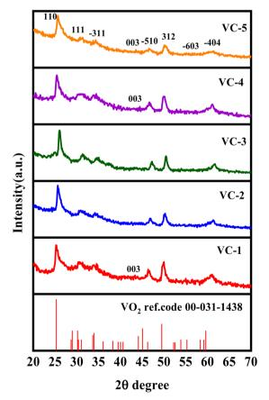
Fig. 1 pXRD pattern of the VO<sub>2</sub>/carbon composites (VC-1 to VC-5).
