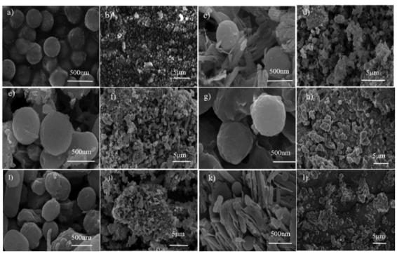
Fig. 2 FESEM images: (a) and (b) carbon, (c) and (d) VO<sub>2</sub>/C-6 h (VC-1), (e) and (f) VO<sub>2</sub>/C-12 h (VC-2), (g) and (h) VO<sub>2</sub>/C-24 h (VC-3) (i) and (j) VO<sub>2</sub>/C-36 h (VC-4), and (k) and (l) VO<sub>2</sub>/C-48 h (VC-5).
