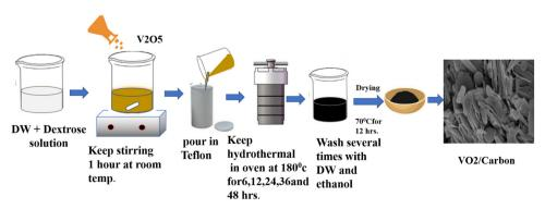
Scheme 1 Schematic diagram of VO<sub>2</sub>/carbon synthesis.
