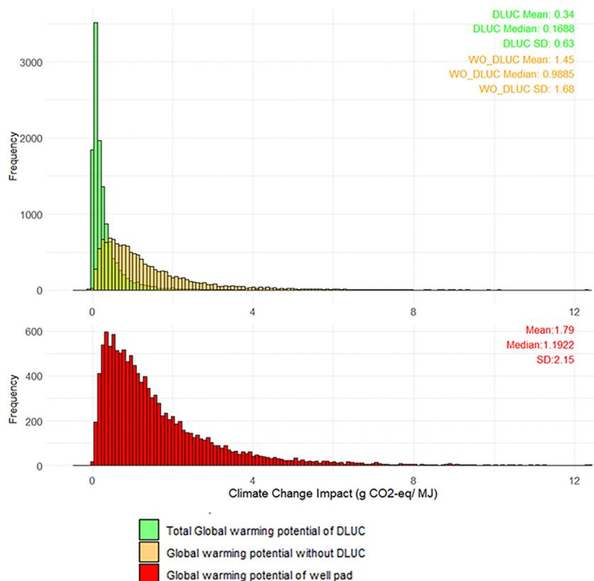
Fig. 3 Global warming potential due to direct land use change (DLUC) impacts and the global warming potential due to other processes (WO\_DLUC) by well pad (top); total global warming impacts of the 12 561 gas well pads including all processes in the bottom histogram.
