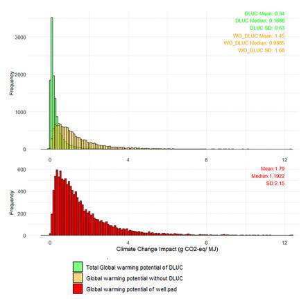
Fig. 3 Global warming potential due to direct land use change (DLUC) impacts and the global warming potential due to other processes (WO\_DLUC) by well pad (top); total global warming impacts of the 12 561 gas well pads including all processes in the bottom histogram.
