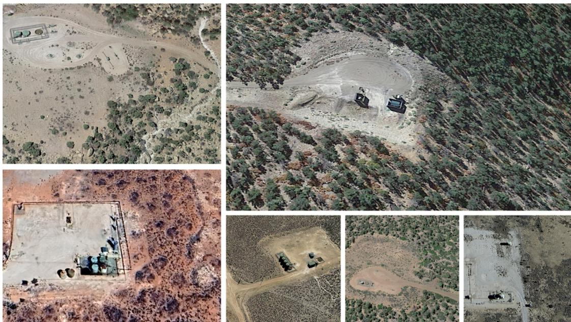
Fig. 1 Examples of natural gas well pads on lands with different types of vegetation (images sourced from Google Maps).
