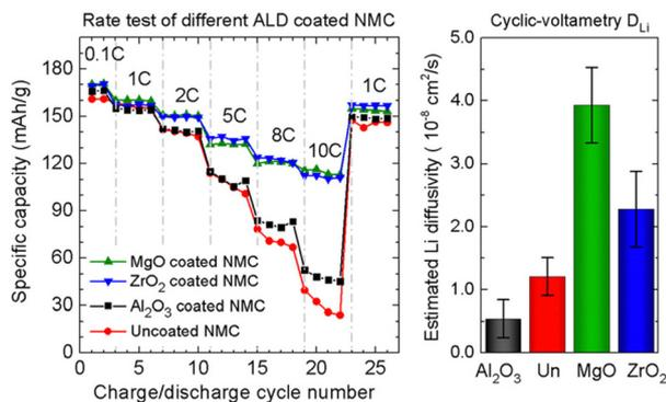
Fig. 6 Rate performance test and Li<sup>+</sup> diffusivity data for uncoated and Al<sub>2</sub>O<sub>3</sub>, ZrO<sub>2</sub>, and MgO-coated NMC532. Reprinted with permission from ref. 124. Copyright 2017 American Chemical Society.
