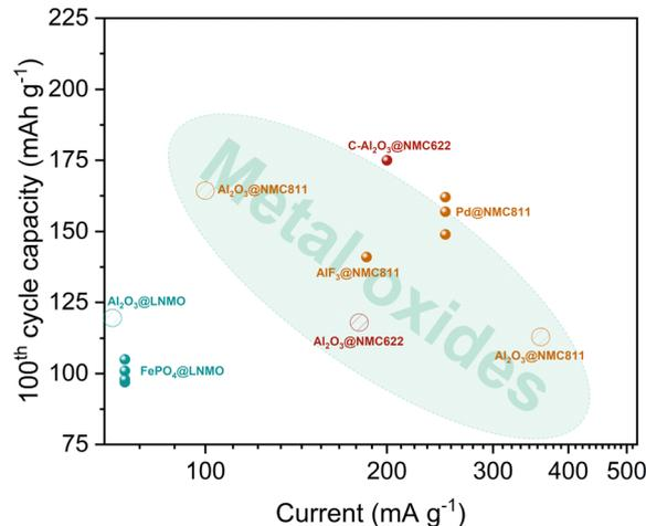
Fig. 10 Specific discharge capacity at the 100th cycle vs. discharge current for CAMs coated with phosphates, fluorides, metals, and organic-derived carbon composites *via* powder ALD. Data points for Al<sub>2</sub>O<sub>3</sub>-coated CAMs are labeled while the highlighted area signifies the best cycling results obtained with metal oxide-based coatings for comparison.
