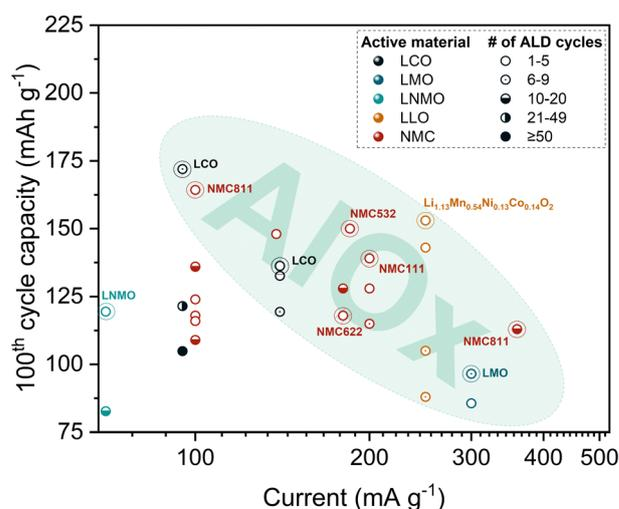
Fig. 3 Specific discharge capacity at the 100th cycle vs. discharge current for intercalation CAMs coated with  $Al_2O_3$  using various number of ALD cycles. Plot is based on cycling data (S1, ESI<sup>†</sup>) using Li metal as counter electrode.
