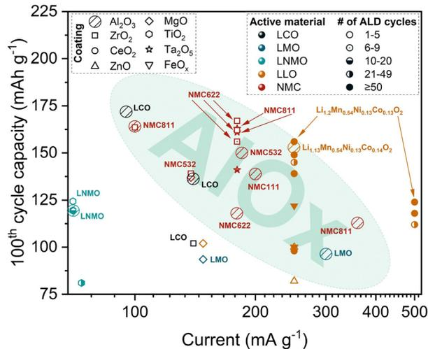
Fig. 5 Specific discharge capacity at the 100th cycle vs. discharge current for CAMs coated with different metal oxides *via* powder ALD. The highlighted area signifies the best cycling results obtained with  $\text{Al}_2\text{O}_3$  coating for comparison.
