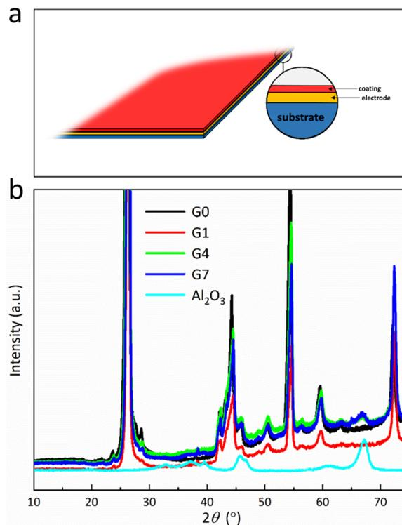
Fig. 2 (a) Illustration of the obtained materials, and (b) XRD spectra of the samples and the raw Al<sub>2</sub>O<sub>3</sub> powder.
