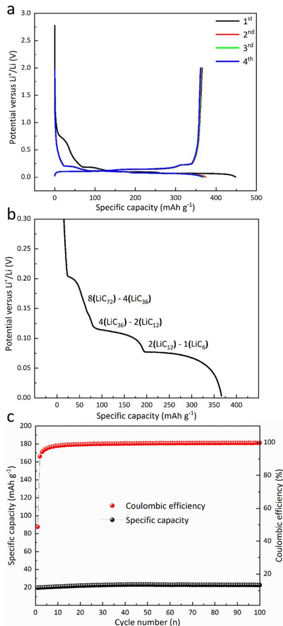
Fig. 1 (a) GDC curves of graphite anodes (cycles 1–4), (b) staging phenomenon (staging information from ref. 21), and (c) cycling performance of the raw material Al<sub>2</sub>O<sub>3</sub> at 75 mA g<sup>-1</sup>.
