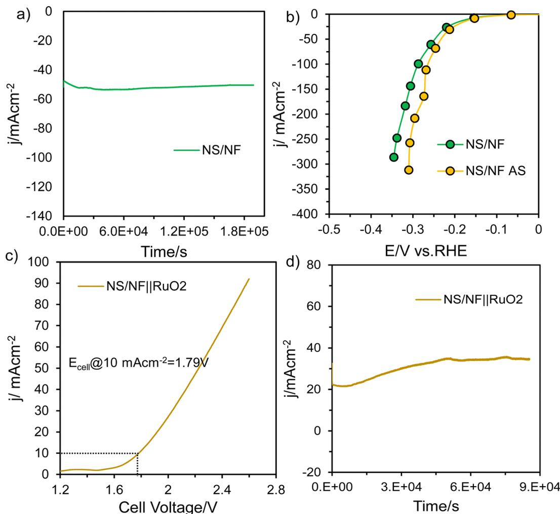
Fig. 5 (a)  $i$ - $t$  curve demonstrating the durability of NS/NF catalyst for HER at a constant potential in  $1.0 \text{ M KOH}$ , (b) SCV curves of NS/NF before and after HER stability, (c) polarisation curves showing overall cell voltage and (d) chronopotentiometry curves for NS/NF||RuO<sub>2</sub> in  $1.0 \text{ M KOH}$ .
