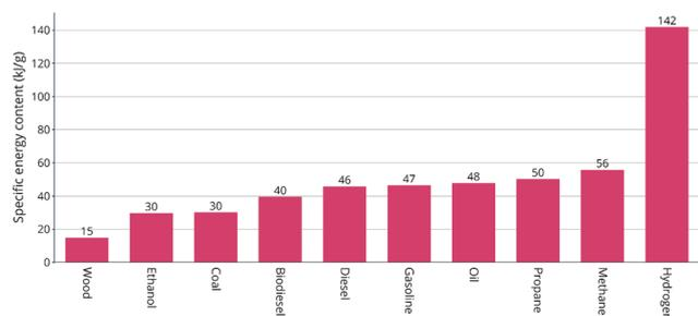
Fig. 5 Specific energy of different fuels (kJ g<sup>-1</sup>).<sup>41</sup>
