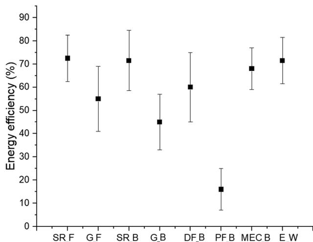
Fig. 4 Average energy efficiency values of H<sub>2</sub> production methods for different resources.<sup>38</sup> SR\_F is steam reforming using fossil, G\_F is gasification using fossil, SR\_B is steam reforming using biomass, G\_B is gasification using biomass, DF\_B is dark fermentation using biomass, PF\_B is photo-fermentation, using biomass, MEC\_B is microbial electrolysis cell using biomass, and E is electrolysis using water.
