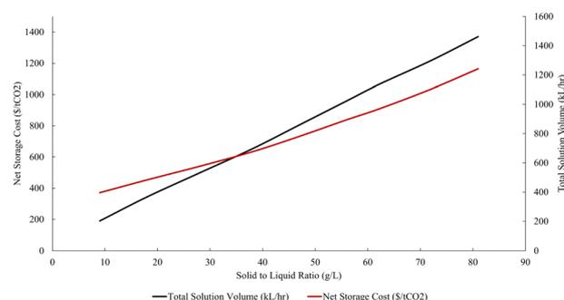
Fig. 4 Effect of increasing solid to liquid ratio on extraction volume and net storage cost.
