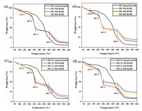
TGA curves of (a) M1, (b) M2, (c) M1 2x and (d) M2 2x for comparison of unactivated and different KOH concentration of activation.
