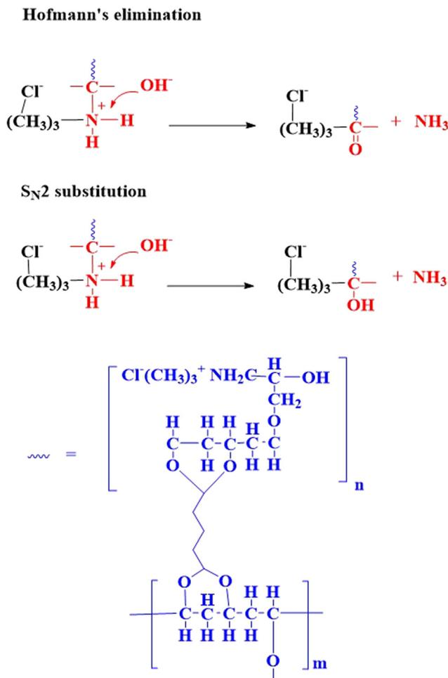
Fig. 8 Hofmann elimination and S<sub>N</sub>2 substitution mechanism in QPVA membranes.
