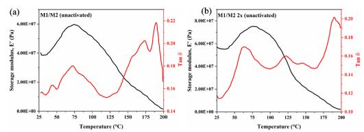
Fig. 6 DMA curve (a) M1/M2 (unactivated) and (b) M1 2x/M2 2x (unactivated) QPVA membranes.
