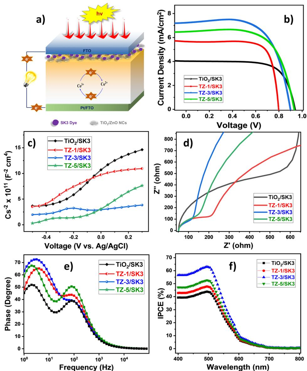
Fig. 1 (a) Schematic of TZ/SK3-based DSSCs. Photovoltaic performance of bare  $\text{TiO}_2/\text{SK3}$ , TZ-1/SK3, TZ-3/SK3, and TZ-5/SK3 NC-based DSSCs: (b)  $I$ - $V$  curves, (c) Nyquist plots, (d) Mott-Schottky plots, (e) Bode phase plot, and (f) IPCE measurement under AM 1.5 G sunlight conditions.
