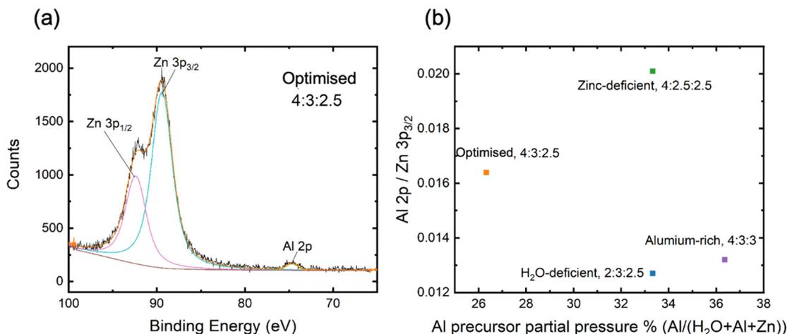
**Fig. 4** (a) Example of fitting of Zn 3p & Al 2p core level peaks in XPS spectra, for optimised case only; (b) Al 2p/Zn 3p<sub>3/2</sub> ratio across annealed, sputter-cleaned samples with the four different pressure profiles, determined from the integrated intensity of Zn 3p<sub>3/2</sub> and Al 2p core peaks, as measured with XPS.
