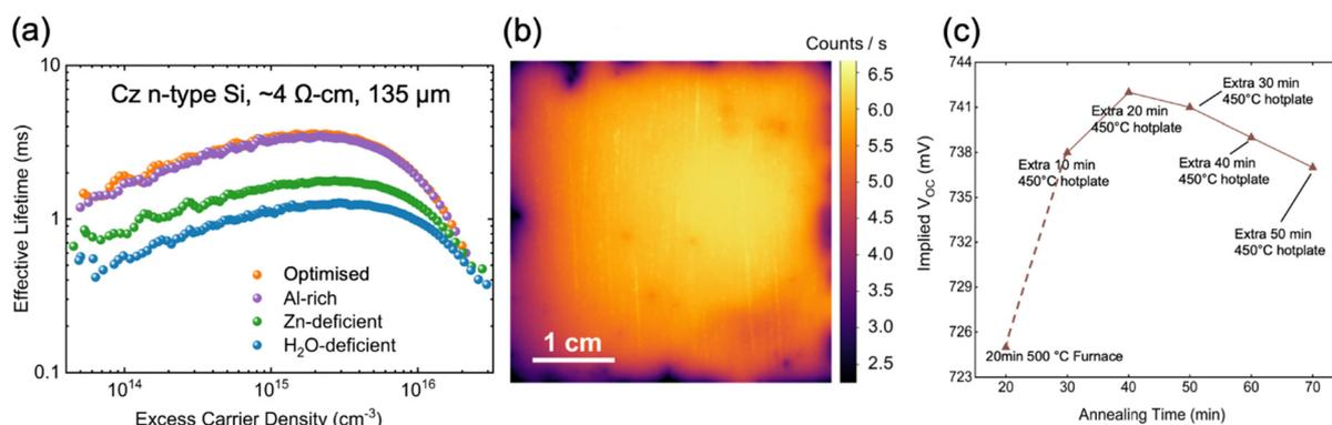
**Fig. 2** (a) Effective lifetime vs. excess carrier density of samples from the four different pressure profiles; (b) PL image of the champion sample from the optimised recipe; (c)  $iV_{OC}$  values vs. annealing time for the champion sample undergoing post-deposition annealing at 450 °C.
