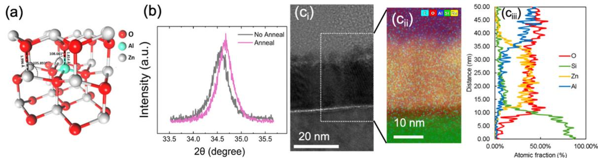
**Fig. 3** (a) Structural model of AZO. (b) XRD spectra of the AZO film in the range of 33.5–35.5° to give insight into the observed peak shift between not annealed and annealed sample; (c) high-resolution high-angle annular dark field (HAADF) TEM image of the crystal structure and defects in AZO; (c<sub>ii</sub>) the enlarged image is the obtained EDS micrograph for a local region of interest. (c<sub>iii</sub>) The averaged EDS has been plotted for elemental analysis of AZO.
