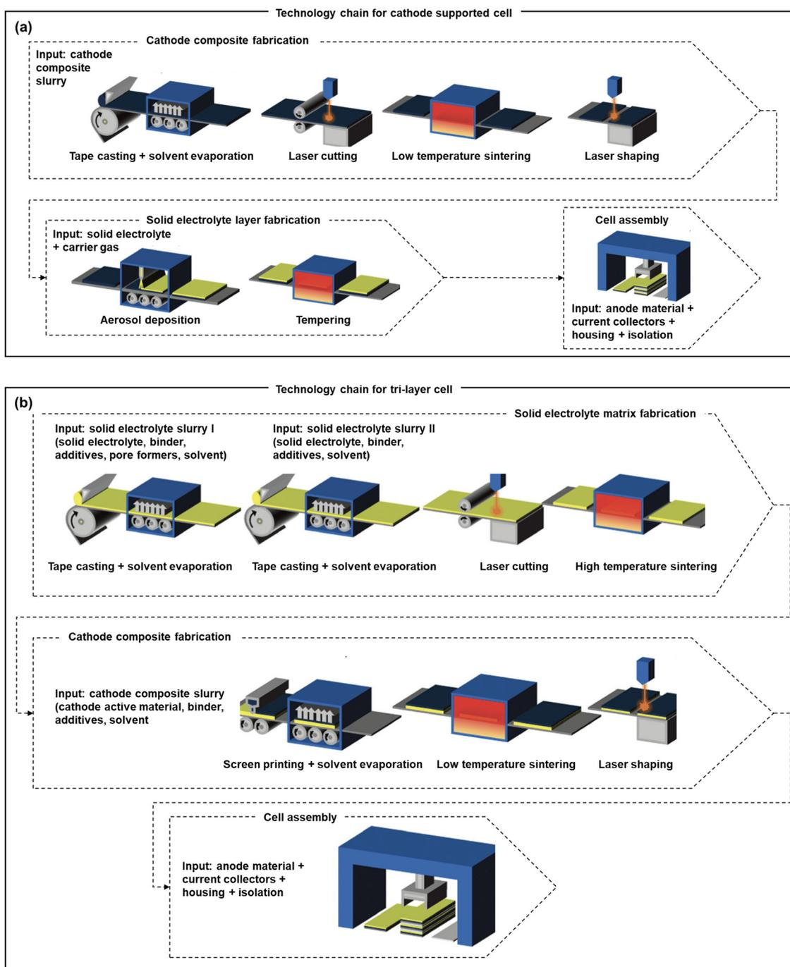
Fig. 11 Examples of manufacturing technology chains for (a) cathode-supported cells and (b) tri-layer cell.<sup>212</sup> (Reproduced with permission from The Royal Society of Chemistry.)
