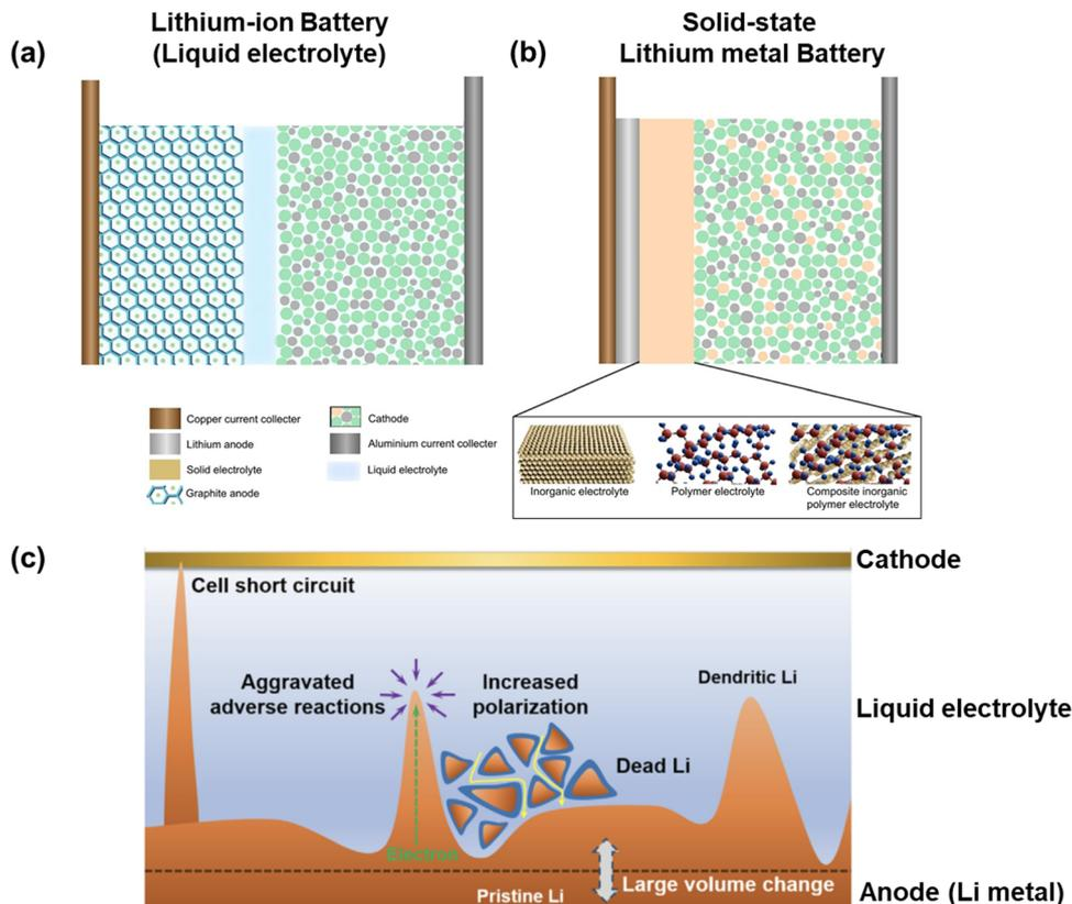
Fig. 1 Schematics of (a) conventional Li-ion battery (LIB) and (b) solid-state Li metal battery (SSLMB);<sup>5</sup> and (c) safety issues with Li-metal anodes in conventional LIB.<sup>10</sup>
