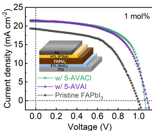
Fig. 6 Forward scan  $J$ - $V$  curves for the champion devices or pristine FAPbI<sub>3</sub>, and FAPbI<sub>3</sub> with 1 mol% 5-AVAI or 5-AVACI added. Inset shows the device structure.
