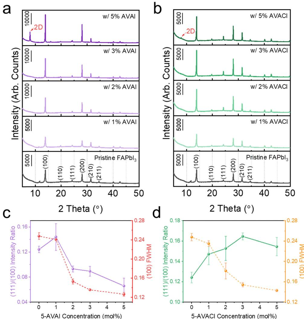
Fig. 3 XRD patterns of the FAPbI<sub>3</sub> films with 1–5 mol% of (a) 5-AVAI and (b) 5-AVACl, and their corresponding (c) and (d) intensity ratios and FWHM.
