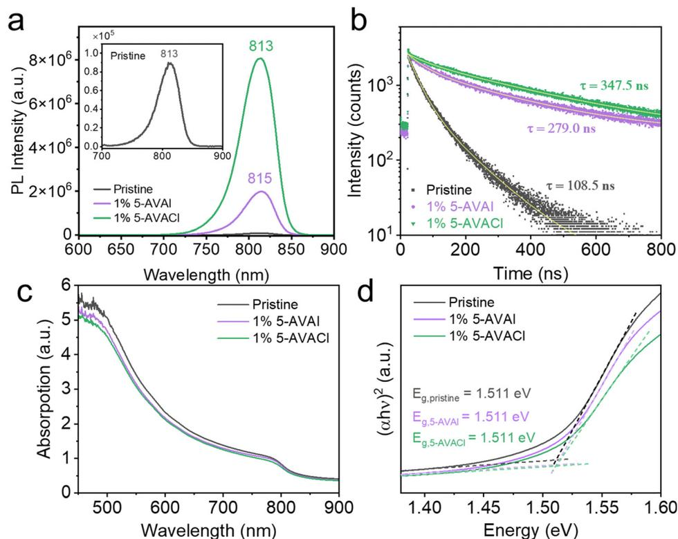
Fig. 5 Optical properties of FAPbI<sub>3</sub> films with and without additives. (a) Steady-state PL and (b) time-resolved PL of pristine FAPbI<sub>3</sub> and FAPbI<sub>3</sub> with 1 mol% 5-AVAI or 5-AVACI. Inset in (a) shows the zoomed-in view of pristine FAPbI<sub>3</sub>. (c) Absorption spectra and (d) Tauc plots of pristine FAPbI<sub>3</sub> and FAPbI<sub>3</sub> with 1 mol% 5-AVAI or 5-AVACI.
