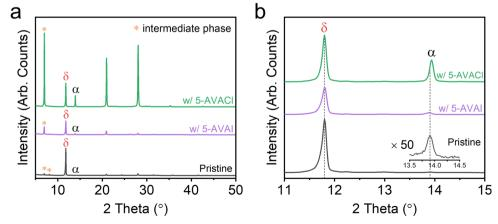
Fig. 4 (a) Full XRD patterns and (b) zoomed-in view of the as-cast FAPbI<sub>3</sub> films without additives and with 5 mol% 5-AVAI or 5-AVACI.
