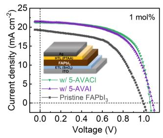
Fig. 6 Forward scan J-V curves for the champion devices or pristine FAPbl<sub>3</sub>, and FAPbl<sub>3</sub> with 1 mol% 5-AVAI or 5-AVACI added. Inset shows the device structure.
