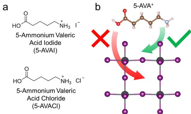
**Fig. 1** (a) Molecular structures of the additives used in this work, 5-AVAI and 5-AVACl. (b) Illustration of a FAPbI<sub>3</sub> lattice (with cations removed) showing that the large 5-AVA<sup>+</sup> cation can fit in the A-sites at the surface, but not within the crystal bulk. Because the 5-AVA<sup>+</sup> cation remains at the surface rather than in the crystal bulk, it does not distort the lattice and cause a deleterious band gap increase.
