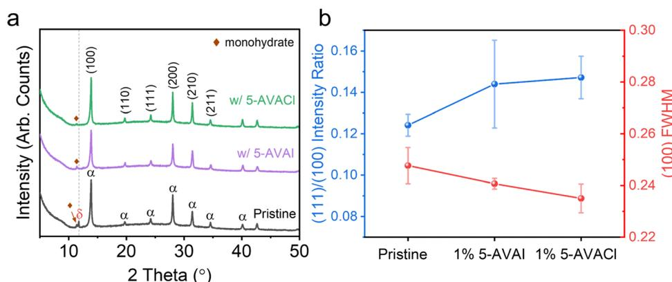
**Fig. 2** (a) XRD patterns of the pristine FAPbI<sub>3</sub> film and the films prepared with 1 mol% 5-AVAI or 5-AVACl. (b) (111)/(100) intensity ratios and FWHM of the (100) peak in FAPbI<sub>3</sub> films with and without additives.
