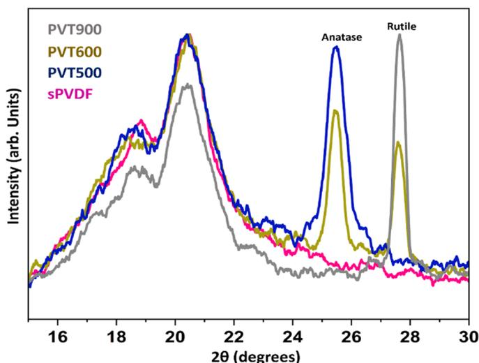
Fig. 6 Comparison of XRD patterns of sPVDF, PVT500, PVT600 and PVT900 in the  $2\theta$  range 15°–30°.
