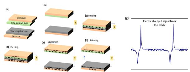
Fig. 9 (a)-(f) Schematic representation of the principle of operation of the contact-separation mode TENG and (g) the electrical output signal obtained from the of the vertical contact-separation TENG tests
