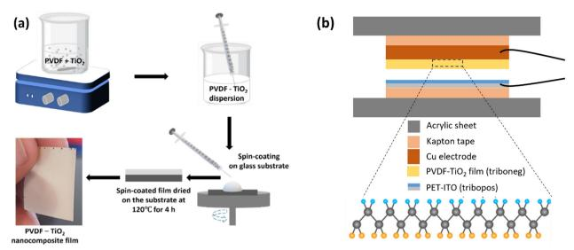
Fig. 1 Schematic representation of (a) the preparation of PVDF-TiO<sub>2</sub> nanocomposite films by spin coating and (b) the design of the fabricated TENG device.
