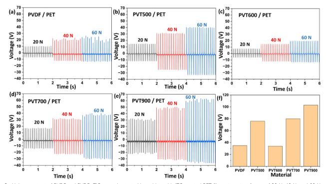
Fig. 8 Voltage output of PVDF and PVDF-TiO2 samples tested by pairing with ITO-coated PET films at contact forces of 20 N, 40 N, and 60 N and a frequency of 8 Hz using a force impactor. (a) Pristine PVDF film, (b) PVT500 film, (c) PVT600 film, (d) PVT700 film, (e) PVT900 film, and (f) graphical comparison of peak-to-peak voltage values
