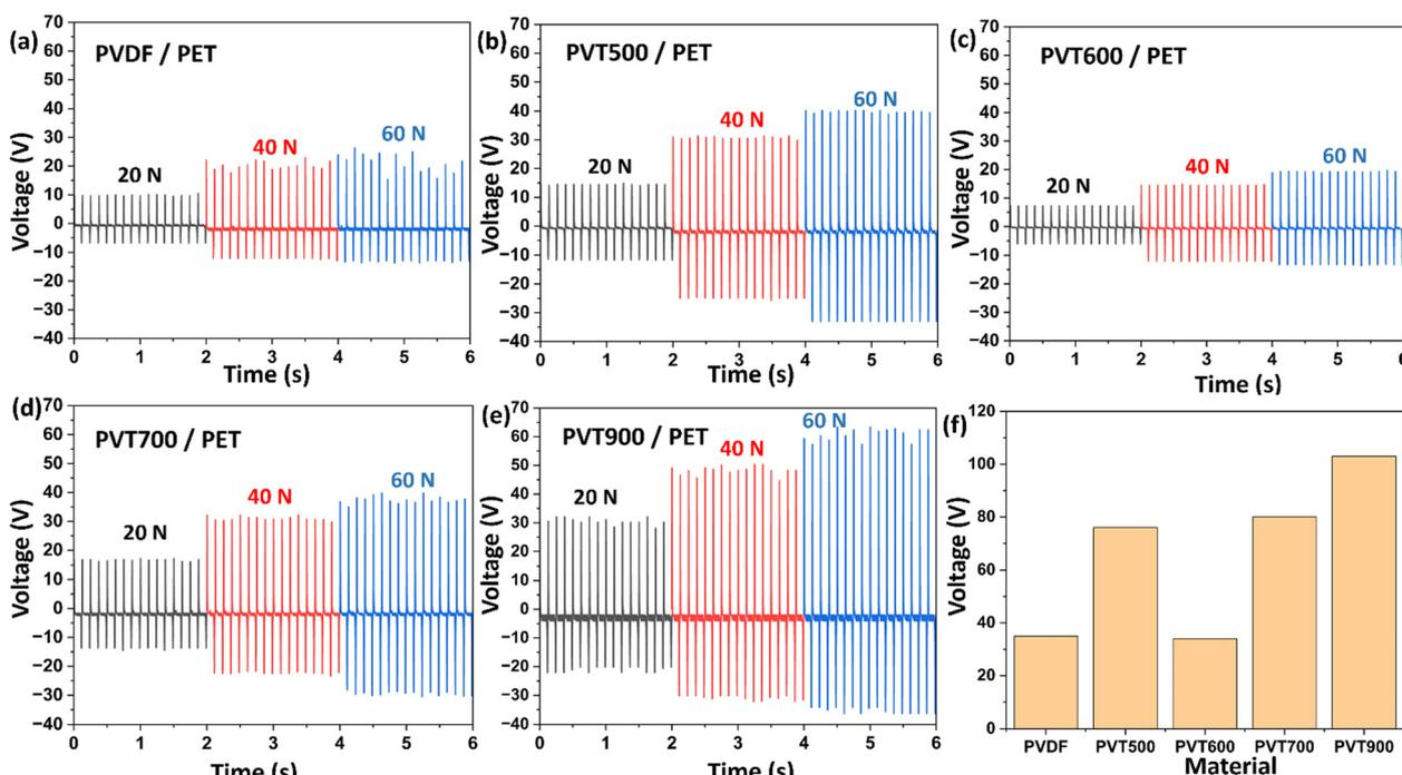
Fig. 8 Voltage output of PVDF and PVDF–TiO<sub>2</sub> samples tested by pairing with ITO-coated PET films at contact forces of 20 N, 40 N, and 60 N and a frequency of 8 Hz using a force impactor. (a) Pristine PVDF film, (b) PVT500 film, (c) PVT600 film, (d) PVT700 film, (e) PVT900 film, and (f) graphical comparison of peak-to-peak voltage values.
