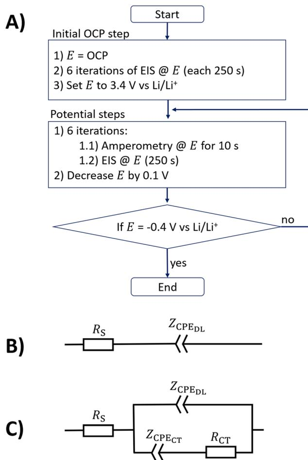
**Fig. 1** (A) Flow chart of the electrochemical step protocol used in this study. (B) Equivalent circuit model of a blocking electrode, consisting of the electrolyte resistance and a constant phase element (CPE) for double layer (DL) capacitance. (C) Equivalent circuit model including the double layer (DL) and a charge transfer (CT) process with transport limitations that are parameterized by a CPE.
