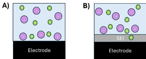
**Fig. 3** Schematic sketch showing the electrochemical interface on the glassy carbon electrode. Green dots: lithium cations. Violet dots: anions. Light blue shading: electrolyte phase. Gray shading: solid electrolyte interphase (SEI). Black: glassy carbon electrode. (A) At the electrode without SEI coverage, the ions are directly adsorbed at the electrode. (B) With SEI coverage, the ion movement is constrained so that ion accumulation and adsorption directly at the electrode are hampered.
