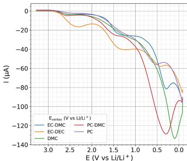
Fig. 5 The first descending branch of cyclic voltammetry (CV) from 3.4 to 0 V vs. Li/Li<sup>+</sup> on different electrolytes.
