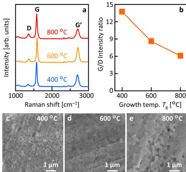
Fig. 2  $T_g$  dependent growth morphologies. (a) Raman spectra obtained from the sample surface. (b) G/D intensity ratio of the samples determined by the Raman spectra shown in (a). SEM images of the samples for  $T_g =$  (c) 400 °C, (d) 600 °C, and (e) 800 °C.
