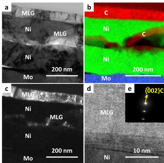
Fig. 3 Characterization of the cross-section of the sample for  $T_g = 400$  °C. (a) Bright-field TEM image. (b) EDX elemental map. (c) Dark-field TEM image using the C(002) plane reflection. (d) High-resolution lattice images showing the lower part of the MLG layer. (e) Selected area electron diffraction pattern taken from the region including MLG with a selected area diameter of 200 nm.
