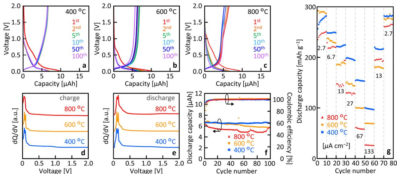
Fig. 4 Anode properties of the samples. Galvanostatic charge/discharge cycles of the samples for  $T_g =$  (a) 400 °C, (b) 600 °C, and (c) 800 °C, where the current density is 13  $\mu\text{A cm}^{-2}$ . dQ/dV plots of (d) charge and (e) discharge for the 10th cycle. (f) Discharge capacity and coulombic efficiency as a function of cycle number. (g) Current-rate testing of the samples at current densities ranged from 2.7 to 133  $\mu\text{A cm}^{-2}$ , every 10 cycles.
