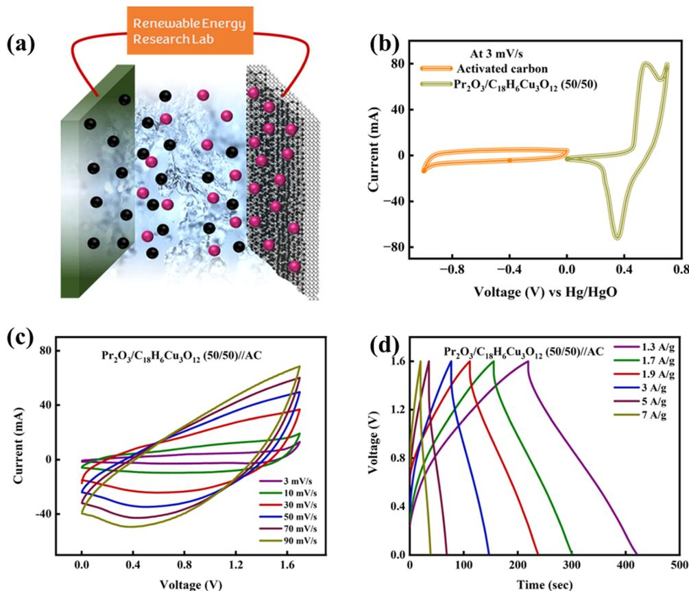
Fig. 6 (a) Schematic of the real device. (b) Comparison of CV curves of activated carbon and  $\text{Pr}_2\text{O}_3/\text{C}_{18}\text{H}_6\text{Cu}_3\text{O}_{12}$  (50/50). (c) Cyclic voltammograms of  $\text{Pr}_2\text{O}_3/\text{C}_{18}\text{H}_6\text{Cu}_3\text{O}_{12}$  (50/50)//AC. (d) Galvanostatic charge–discharge curves of  $\text{Pr}_2\text{O}_3/\text{C}_{18}\text{H}_6\text{Cu}_3\text{O}_{12}$  (50/50)//AC.
