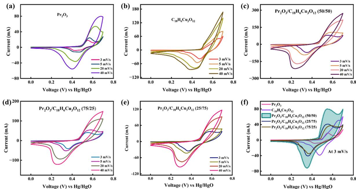
Fig. 3 Cyclic voltammograms of (a)  $\text{Pr}_2\text{O}_3$ , (b)  $\text{C}_{18}\text{H}_6\text{Cu}_3\text{O}_{12}$ , (c)  $\text{Pr}_2\text{O}_3/\text{C}_{18}\text{H}_6\text{Cu}_3\text{O}_{12}$  (50/50), (d)  $\text{Pr}_2\text{O}_3/\text{C}_{18}\text{H}_6\text{Cu}_3\text{O}_{12}$  (75/25), and (e)  $\text{Pr}_2\text{O}_3/\text{C}_{18}\text{H}_6\text{Cu}_3\text{O}_{12}$  (25/75). (f) Comparison of all the samples' voltammograms at  $3 \text{ mV s}^{-1}$ .
