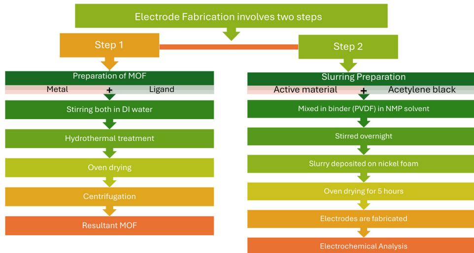
Fig. 1 Synthesis of MOFs and the fabrication process of electrodes.
