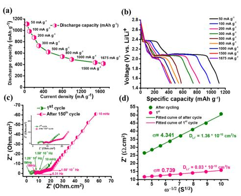
Fig. 5 (a) and (b) Rate capability plot at different current densities. (c) EIS spectra of RRGO-S@CF for the 1st and 150th cycle (cycling at 200 mA g<sup>-1</sup>) with their frequencies. (d) Plot of Z' vs.  $\omega^{-1/2}$  ( $S^{1/2}$ ) in the low-frequency region.
