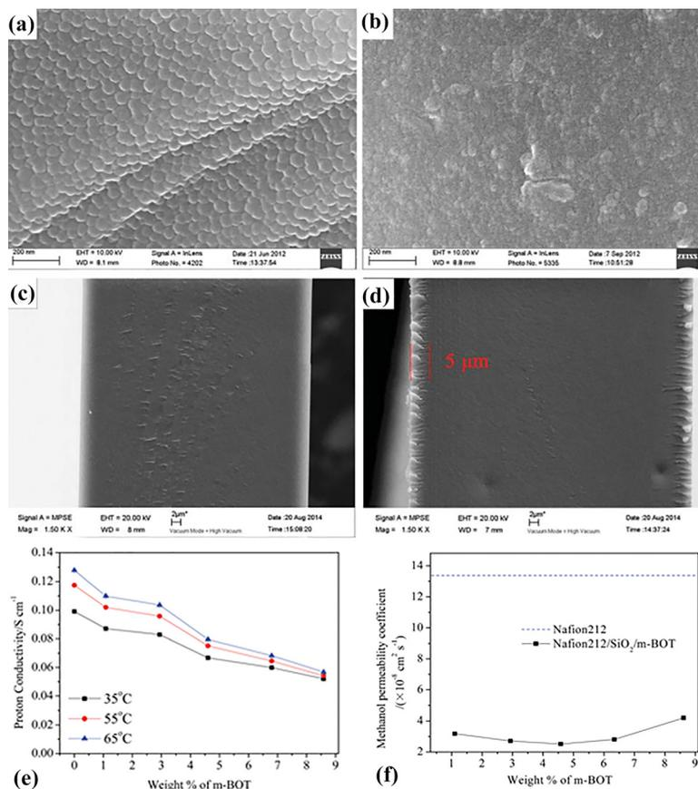
Fig. 6 The SEM images of the top surface (a) and cross section (c) of the Nafion 212 membrane. (b) Top surface and (d) cross section of the Nafion/SiO<sub>2</sub>/m-BOT composite membrane. (e) Different amounts of the m-BOT based composite membrane vs. proton conductivity at 35 °C, 55 °C and 65 °C. (f) Different amounts of the m-BOT based composite membrane vs. methanol permeability values at 25 °C.<sup>91</sup> With copyright permission, 2018, American Chemical Society.
