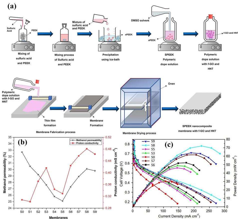
**Fig. 13** Schematic diagram of the preparation process of sulfonated SPEEK incorporated with functionalized graphene oxide and HNT. (b) Pristine and SPEEK nanocomposite membranes with f-GO and HNT vs. methanol permeability and proton conduction values. (c) Current density vs. cell voltage and power density curves for different types of membranes with and without F-GO and HNT based membranes in a DMFC single cell.<sup>174</sup> With copyright permission, 2022, Elsevier.
