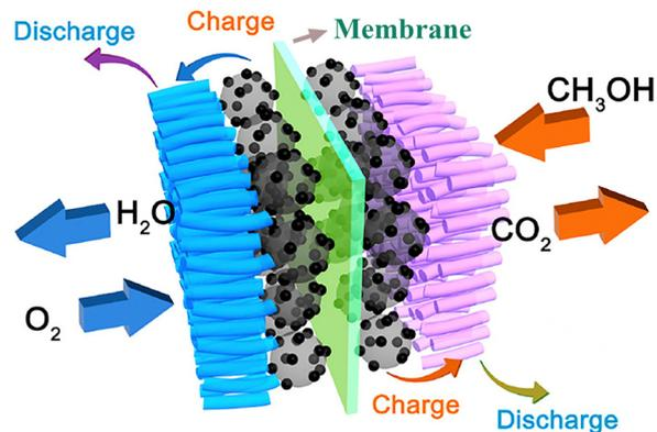
Fig. 1 Schematic diagram of the DMFC mechanism.<sup>16</sup> With copyright permission, 2018, American Chemical Society.
