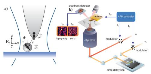
Fig. 13 Photoinduced interaction and configuration of PiFM. Reproduced with permission.<sup>381</sup> Copyright 2015, the American Chemical Society. (a) Representation of the interaction between the photoinduced tip dipole in the focal plane of a tightly focused field and in the target particle. (b) Configuration of the PiFM.
