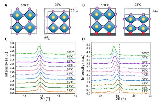
Fig. 11 Process of strain formation. The positive thermal expansion coefficient (A-B), intensity vs. temperature (C-D). Reproduced with permission.<sup>56</sup> Copyright 2017, American Association for the Advancement of Science.
