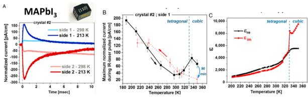
Fig. 9 Relative permittivity and pyroelectric response measurements. (a) Pyroelectric response,  $J_{\text{pyro}}$ , in the direction of  $\langle 001 \rangle$ , (b) the pyroelectric character of MAPbl<sub>3</sub> derived from the peak-current value reliance on temperature. Reproduced with permission.<sup>321</sup> Copyright 2011, Macmillan Publishers Limited
