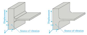
Fig. 18 Cross-sections of the beam in generators. Reproduced with permission.<sup>432</sup> Copyright 2010, Proceedings of PowerMEMS.
