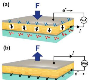
Fig. 16 Hybrid perovskite piezoelectric nanogenerator structure. (a) Electrons move from the top electrode to the bottom electrode side (b) collected electrons from the bottom electrode flow back to the top electrode. Reproduced with permission.<sup>14</sup> Copyright 2016, WILEY-VCH Verlag GmbH & Co. KGaA, Weinheim.
