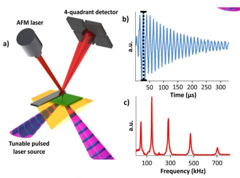
Fig. 14 Instrumentation: reproduced with permission. 404 Copyright 2013, the American Chemical Society. (a) Picture of the PTIR technique, (b) high peak to peak deflection and (c) amplitude of different contact resonance modes.
