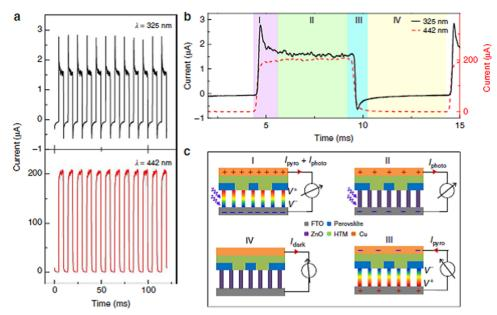
Fig. 21 Working mechanism of self-powered ZPH PDs. Reproduced with permission. 331 (a) I-t curves for self-powered ZPH photodetectors, (b) Lightself-induced pyro-electric effect, (c) the pyro-potential distribution. Copy right 2015 Macmillan Publishers Limited.
