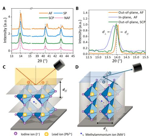
Fig. 1 Characterization of halide perovskite strain property. (A) crystal pattern, (B) plane orientation, (C) the out-of-plane XRD and (D) in-plane XRD. Reprinted with permission.<sup>56</sup> Copyright 2017, American Association for the Advancement of Science
