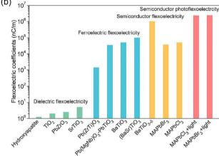
Fig. 22 Photoflexoelectricity: reproduced with permission. 474 Copyright 2020. Nature Publishing Group. (a) Polarization of MAPbBr<sub>3</sub> upon bending in the dark and presence of light and (b) flexoelectric coefficients of various perovskite oxides and halides
