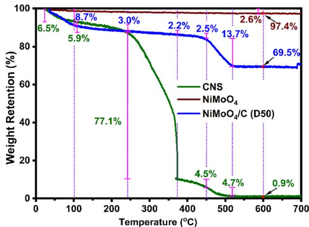
Fig. 4 TGA profiles of CNS, NiMoO<sub>4</sub>, and NiMoO<sub>4</sub>/C (D50).
