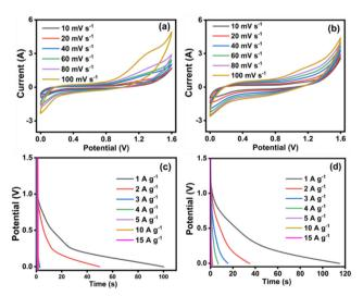
Fig. 15 The electrochemical performances of NiMoO<sub>4</sub>/C (D50) based symmetric (left) and asymmetric (right) SCs: (a) and (b) CV curves at different scan rates, and (c) and (d) GCD curves at different current densities.
