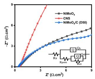
Fig. 13 EIS Nyquist plot of NiMoO<sub>4</sub>, CNS and NiMoO<sub>4</sub>/C (D50) samples with the inset of their equivalent circuit.
