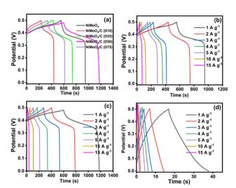
Fig. 10 GCD curves at different current densities: (a) comparison data of NiMoO<sub>4</sub> and NiMoO<sub>4</sub>/C (Dx) at 1 A  $g^{-1}$ , (b) NiMoO<sub>4</sub>, (c) NiMoO<sub>4</sub>/C (D50) and (d) CNS
