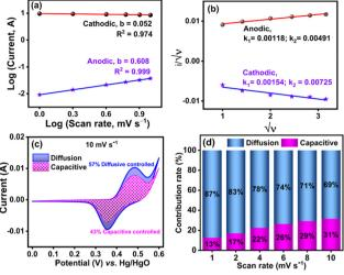
Fig. 14 Kinetics of energy storage behavior of NiMoO<sub>4</sub>/C (D50) at different scan rates (1–10 mV s<sup>-1</sup>): (a) plot of  $\log(i)$  vs.  $\log(v)$ , (b) plot of  $i/\sqrt{\nu}$  and  $\sqrt{\nu}$  (c) CV cycles of capacitive-contribution (pink-shaded region) and diffusion-contribution (blue-shaded region) at 10 mV s<sup>-1</sup>, and (d) total contribution rate of capacitive (pink) and diffusion-controlled (blue) processes at different scan rates
