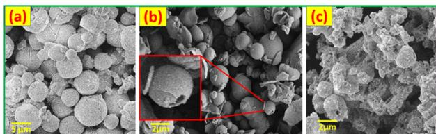
Fig. 5 FESEM images of (a)  $\text{NiMoO}_4$ , (b) CNS and (c)  $\text{NiMoO}_4/\text{C}$  (D50).
