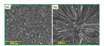
Fig. 12 FESEM images of the NiMoO<sub>4</sub>/C (D50) electrode (a) before and (b) after cyclic stability studies performed for GCD 5000 cycles at 5 A g<sup>-1</sup>
