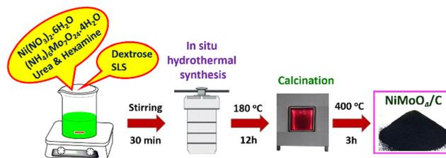
Scheme 1 Schematic representation of *in situ* hydrothermal synthesis of the NiMoO<sub>4</sub>/C nanocomposite.
