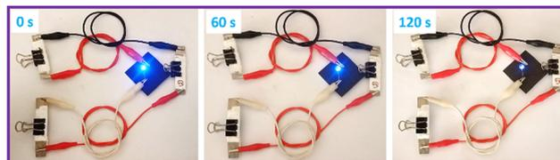
Fig. 16 Demonstration of powering a blue LED light by three NiMoO<sub>4</sub>/C (D50) based symmetric SC devices connected in series.
