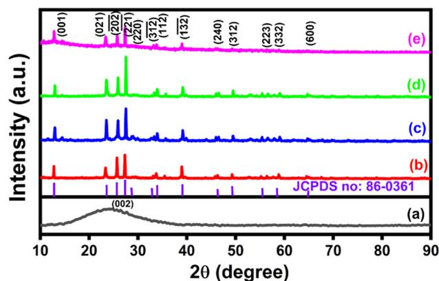
Fig. 1 XRD patterns of (a) CNS, (b) NiMoO<sub>4</sub>, (c) NiMoO<sub>4</sub>/C (D25), (d) NiMoO<sub>4</sub>/C (D50) and (e) NiMoO<sub>4</sub>/C (D75).
