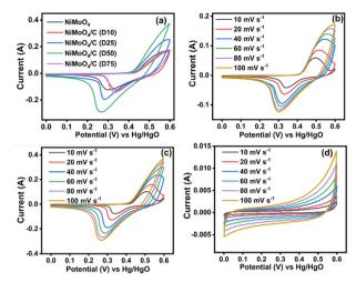
Fig. 9 CV curves at different scan rates: (a) comparison data of NiMoO<sub>4</sub> and  $NiMoO_4/C$  (Dx) at 100 mV s<sup>-1</sup>, (b)  $NiMoO_4$ , (c)  $NiMoO_4/C$  (D50) and (d) CNS.
