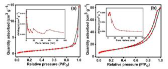
Fig. 7 N<sub>2</sub> adsorption-desorption BET isotherms with corresponding BJH pore-size distributions plots (insets): (a) NiMoO<sub>4</sub> and (b) NiMoO<sub>4</sub>/C (D50).
