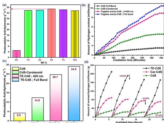
Fig. 3 (a) Cumulative hydrogen generation for different ratios of *Tagetes erecta*-CdS. (b) Cumulative hydrogen generation versus irradiation time for CdS and *Tagetes erecta*-CdS using the full-band solar spectrum and 420 nm wavelength. (c) Photocatalytic activity. (d) Recyclability analysis.
