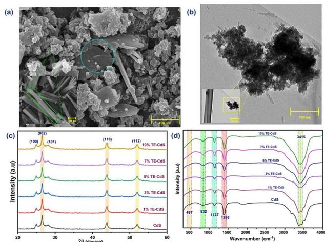
**Fig. 1** FE-SEM micrograph images of (a) *Tagetes erecta*-CdS and CdS nanorod (inset). (b) TEM images of *Tagetes erecta*-CdS and CdS nanorod (inset). (c) XRD analysis of CdS and various concentrations of *Tagetes erecta*-CdS. (d) FTIR analysis of CdS and various concentrations of *Tagetes erecta*-CdS.
