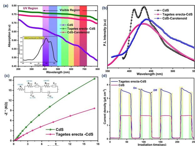
**Fig. 2** (a) UV-vis spectra of CdS and *Tagetes erecta*-CdS. (b) Photoluminescence spectra. (c) EIS spectra of CdS and *Tagetes erecta*-CdS. (d) Transient photocurrent of pure CdS and *Tagetes erecta*-CdS under simulated light.
