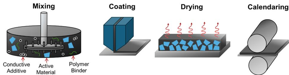
Fig. 1 Illustration of the battery electrode manufacturing process.
