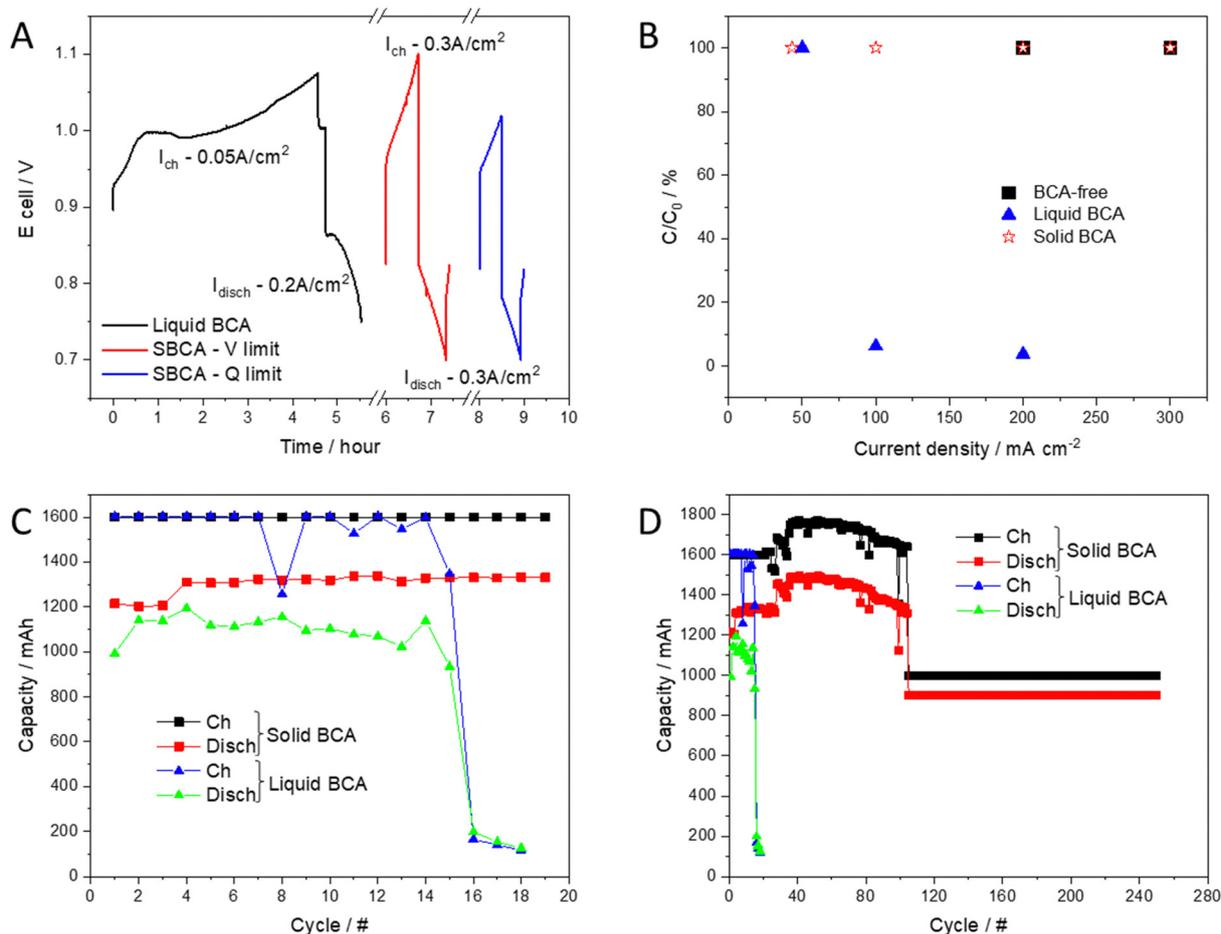
Fig. 4 (A) voltage profile of cell with liquid BCA and SBCA, (B) Ratio of the capacity  $C$  vs. initial capacity  $C_0$  as a function of cycling current density for BCA-free, liquid and solid BCA, (C) and (D) Galvanostatic cycling with liquid BCA and SBCA.
