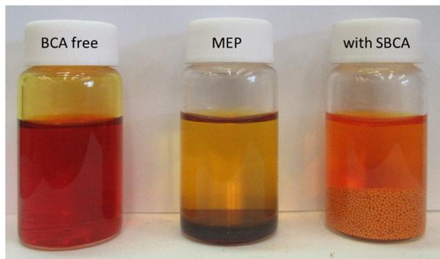
Fig. 1 HBr 6.6 M electrolyte (SoC 66%) without (right) and with liquid (center) and solid (right) BCA.
