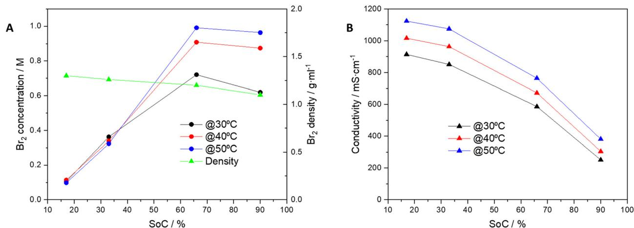
Fig. 2 Dependence on SoC at 30, 40 and 50 °C with SBCA for (A) Br<sub>2</sub> concentration and electrolyte density and (B) electrolyte ionic conductivity.
