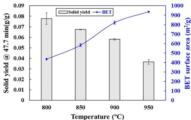
Fig. 9 Yield and surface area of char from PET gasification with CO<sub>2</sub> at different reaction temperatures (reprinted with permission from ref. 69 Copyright 2020 Elsevier).
