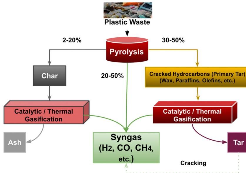
Fig. 3 Flowchart of plastic gasification.
