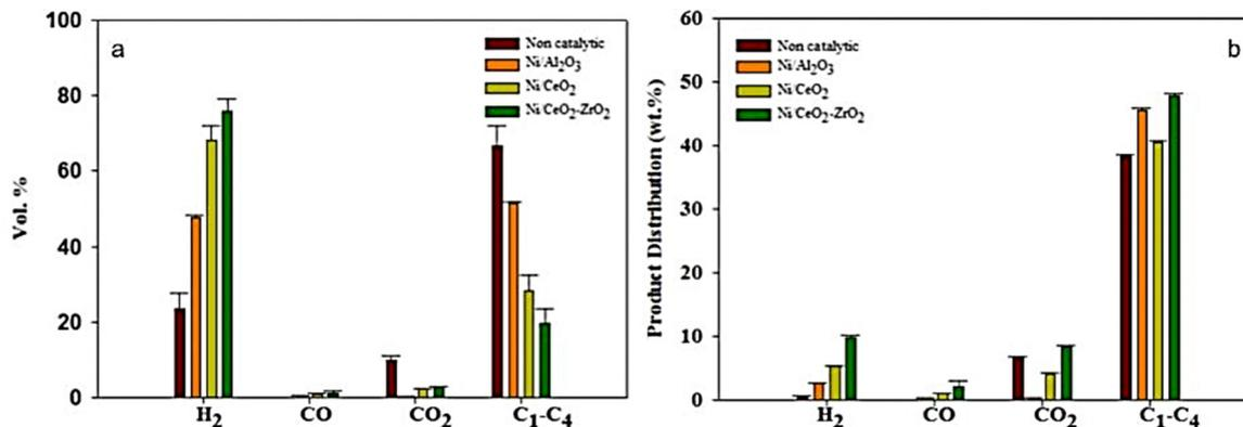
Fig. 17 Effect of Ni/CeO<sub>2</sub>-ZrO<sub>2</sub> catalyst on (a) gas selectivity (vol%) and (b) product distribution (wt%) (reprinted with permission from ref. 138 Copyright 2021 Elsevier).
