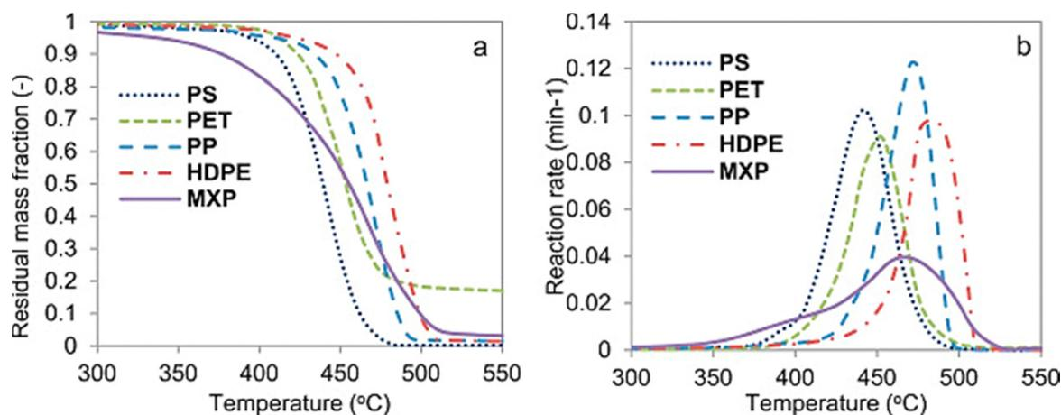
Fig. 10 (a) the plot of residual mass fraction vs. temperature curve and (b) the plot of reaction rate vs. temperature curve at 20 °C min<sup>-1</sup> for individual and mixed plastic waste (reprinted with permission from ref. 30 Copyright 2019 Elsevier).
