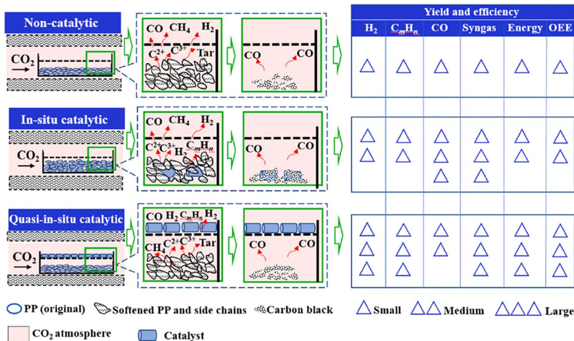
Fig. 14 Comparison of yield and efficiency of CO<sub>2</sub>-assisted gasification of PP among the different catalytic methods (reprinted with permission from ref. 103 Copyright 2021 Elsevier).
