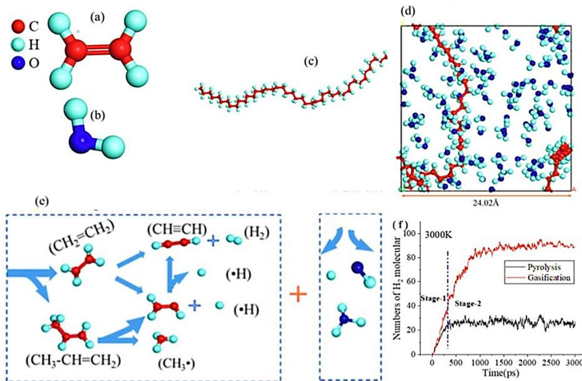
Fig. 6 Steam gasification DFT method: (a) ethylene molecule; (b)  $H_2O$  molecule; (c) the chain of optimized PE; (d) gasification system; (e) depolymerization and steam reforming reaction; (f) distribution of  $H_2$  in gasification (adapted with permission from ref. 54 Copyright 2022 Elsevier).
