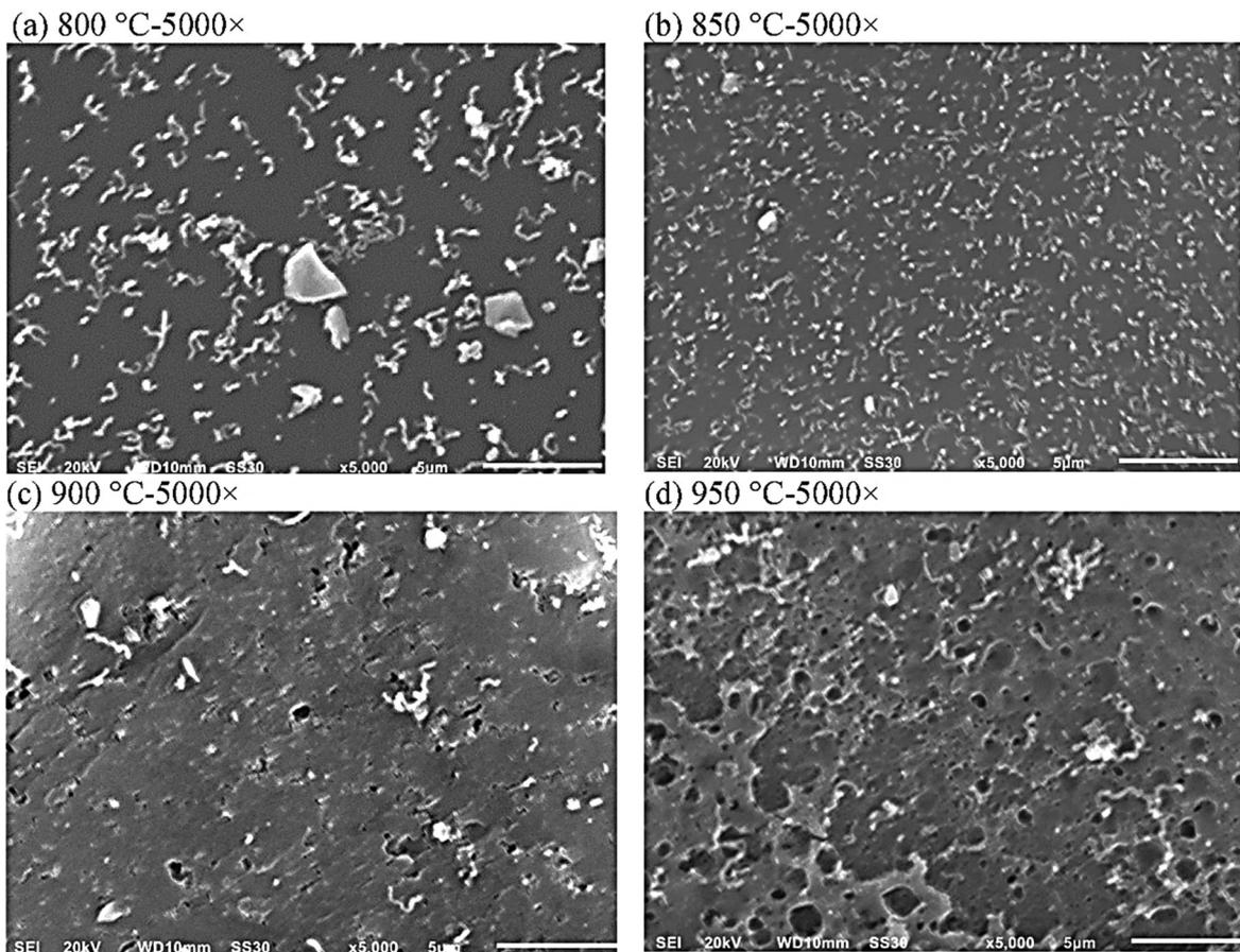
Fig. 8 The morphologies of solid residues of PET gasification with CO<sub>2</sub> at different temperatures: (a) 880 °C, (b) 850 °C, (c) 900 °C, and (d) 950 °C (reprinted with permission from ref. 69 Copyright 2020 Elsevier).
