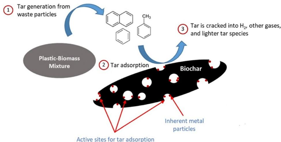
Fig. 16 Mechanisms of tar reforming on biochar during gasification (reprinted with permission from ref. 130 Elsevier 2020 (CC-BY 4)).
